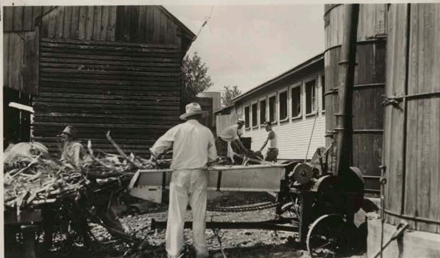
Cutting ensilage with 5 H. P. electric motor on farm in Botetourt County. Five farmers cooperated in the use of this motor for ensilage cutting.
