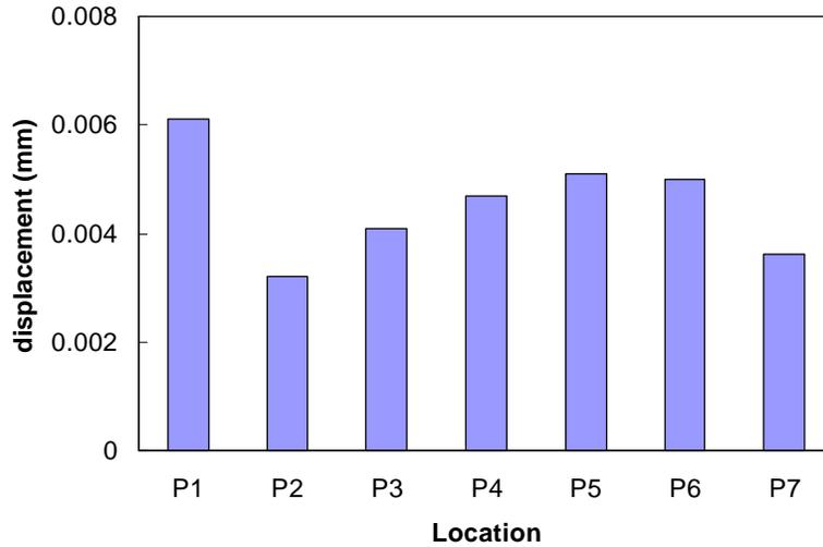
Figure 4.17. Displacement of flex at different locations during temperature cycle of 50°C and 150°C.
