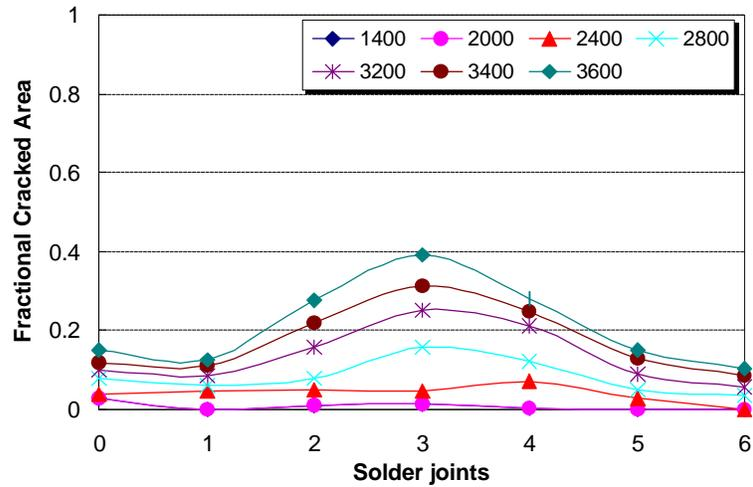
Figure 4.7. The fractional crack area of solder joint and chip pad interface for the seven solder joints on the FCOF assembly at different temperature cycles.
