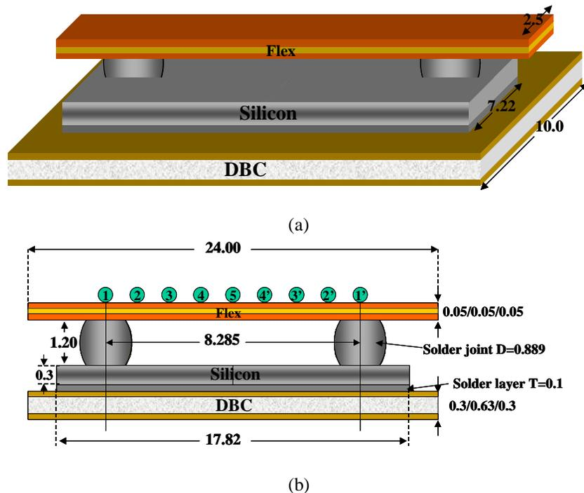
Figure 4.9. Schematic drawing of the one-dimensional flex strip sample. (a) 3-D drawing; (b) cross section.
