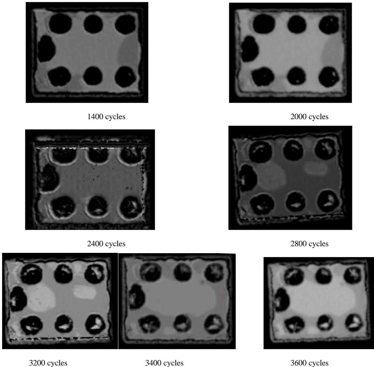
Figure 4.6. Typical C-SAM images of the interface between stacked hourglass/column-shaped solder joints and chip in FCOF assembly during temperature cycling.
