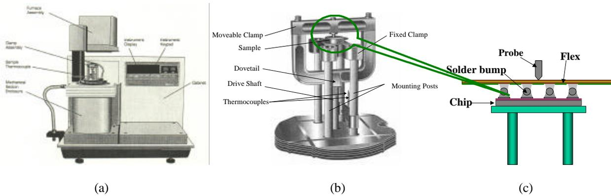
Figure 4.11. The TA Instruments Dynamic Mechanical Analyzer [1]. (a) The outlook; (b) Clamp assembly; (c) Magnified picture of probe and sample under test.
