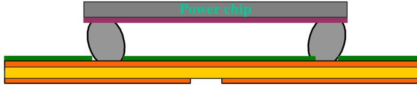
Figure 4.19. Schematic of exaggerated thermal displacements in flip chip on rigid board package.
