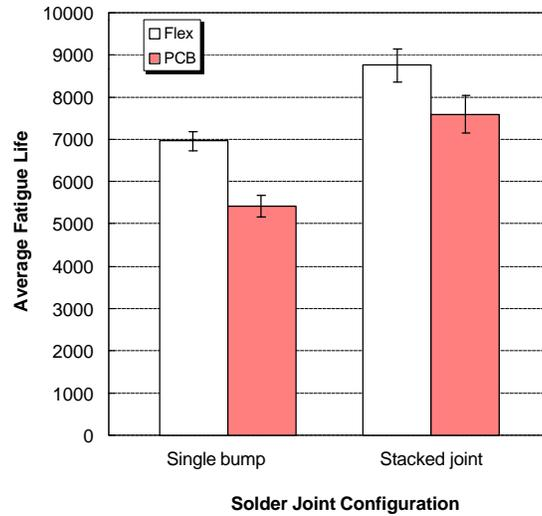
Figure 4.2. A comparison of the average fatigue life of flip chip on PCB board and flip chip on flex assemblies with single bump barrel-shaped solder joints and stacked hourglass/column-shaped solder joints under the first thermal cycling condition.
