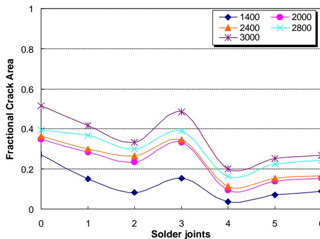
Figure 4.5. The fractional crack area of solder joint and chip pad interface for the seven solder joints on the FCOF assembly at different temperature cycles.
