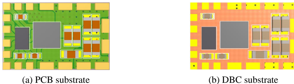
Fig. 3.18: PCB & DBC substrate for single phase modules
