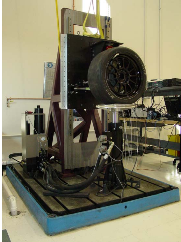
Figure 4-1 Virginia Tech PERL tire coupled quarter-car suspension test rig
