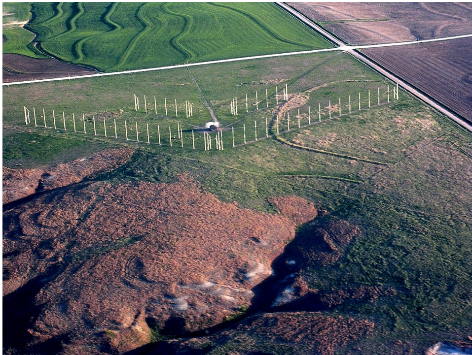
Figure 1.8: A photograph taken from an aircraft showing the layout of the Fort Hays, Kansas SuperDARN radar. The image was taken from the front of the radar looking southwards, with the interferometry arrays visible 100m behind the main arrays. The site features two radars, which view different azimuthal regions. The poles visible are the aluminum support structures which the wire antennas are mounted on. A control building, which houses radar electronics, is in the center.
