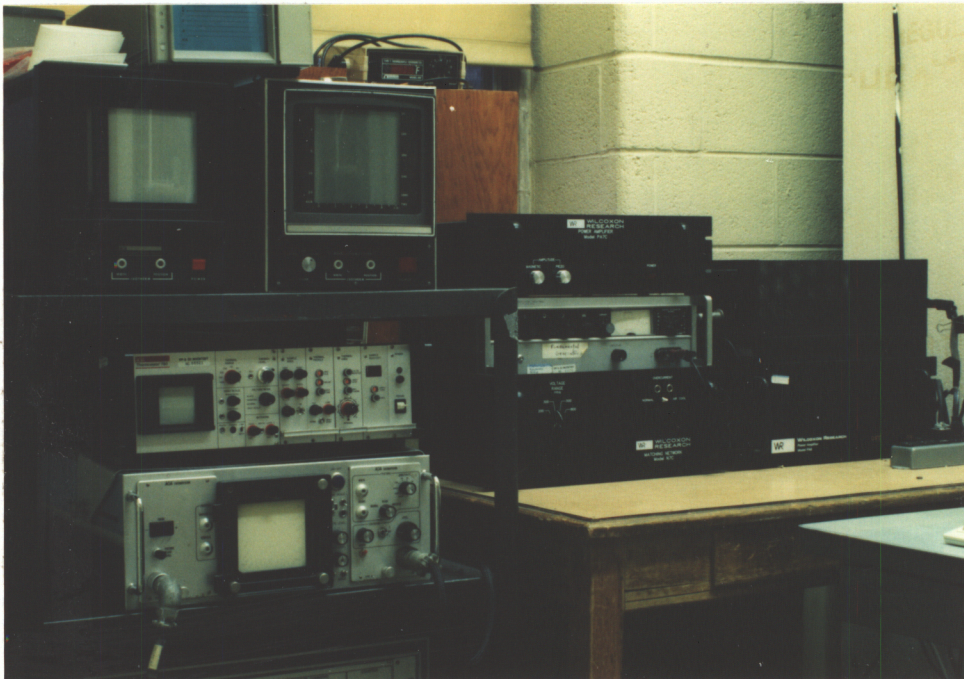
Figure 2. Equipment used for testing. (a) Vibration shaker and thermographic camera; (b) Frequency generator, power amplifiers and display monitors.
