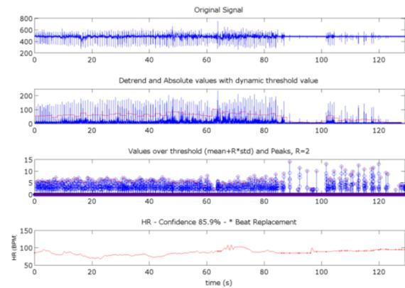
**Figure 4. Stages of the HRtool on an ECG signal.**
