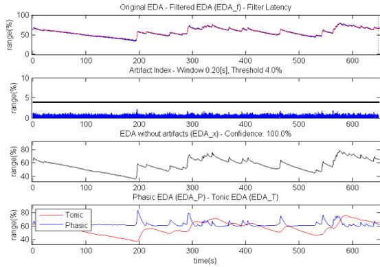
**Figure 2. Stages of the EDAtool on an electrodermal signal.**
