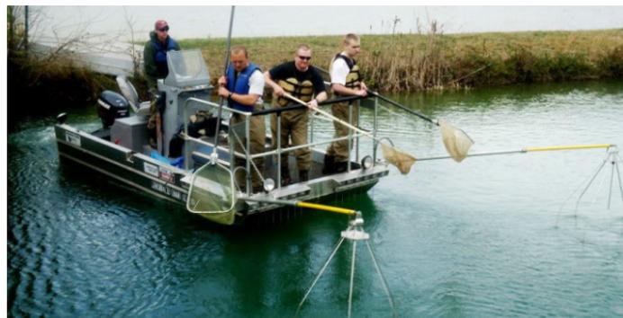
*Students sampled fish using an electrofisher, which uses an electrical current to stun fish.*
