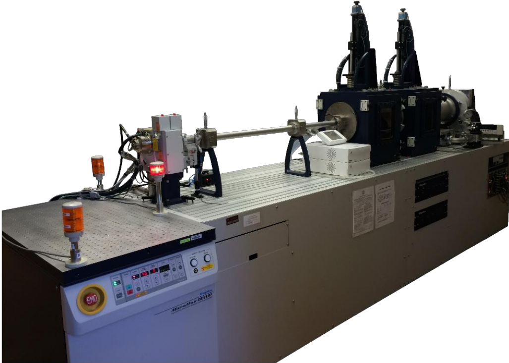
Figure 1.15 Rigaku S-Max 3000 Small and Wide Angle Scattering system in the Moore research group at Virginia Tech
