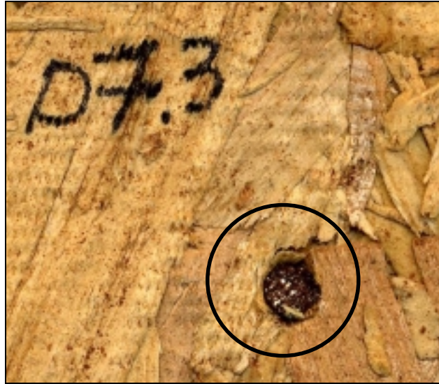
Figure 4.36: Mode III m failure of sample D7-3 (40 cycles).
