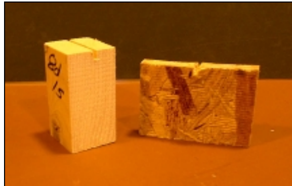
Figure 4.11: Main and side member embedment samples (post-test).
