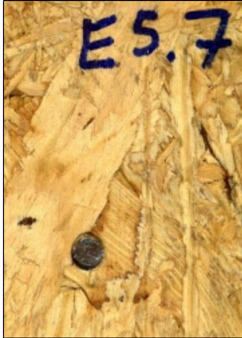
Figure 4.45: Mode III m failure of sample E5-7 (15 cycles).
