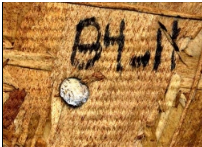
Figure 4.17: Mode III m failure of sample B4-11 (10 cycles).
