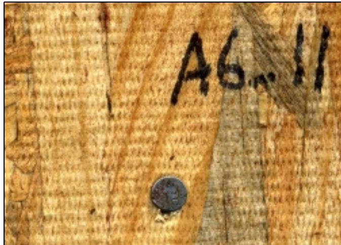
Figure 4.6: Mode III m failure of sample A6-11 (25 cycles).
