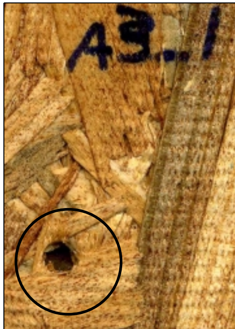
Figure 4.8: Mode III s failure of sample A3-1 (5 cycles).
