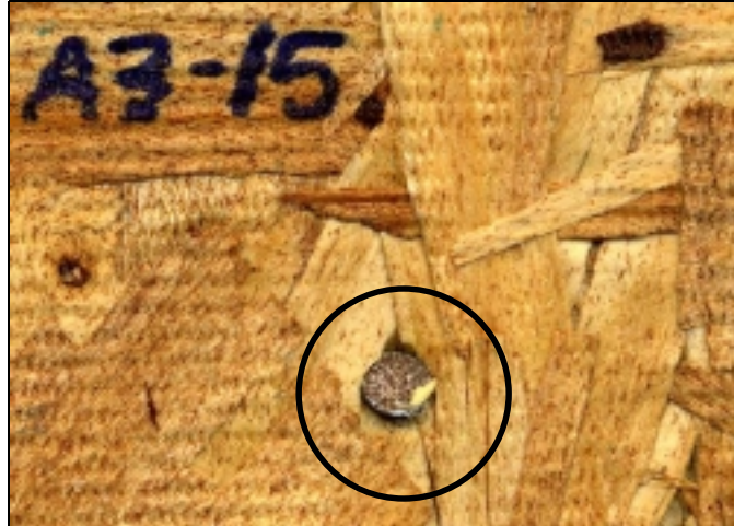
Figure 4.7: Mode III m failure of sample A3-15 (5 cycles).
