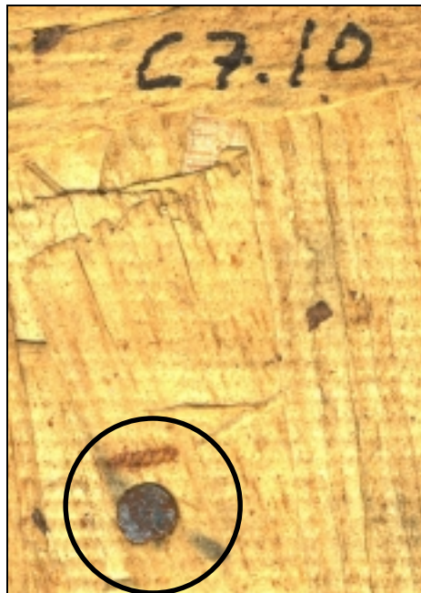
Figure 4.26: Mode III m failure of sample C7-10 (40 cycles).
