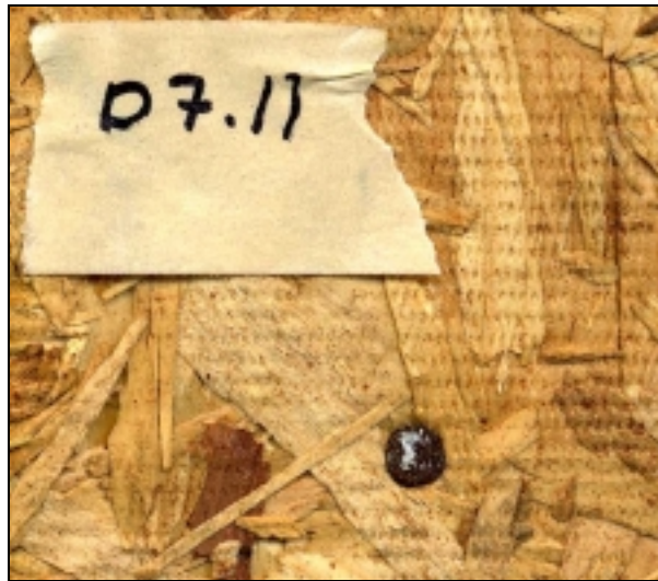
Figure 4.35: Mode III m failure of sample D7-11 (40 cycles).
