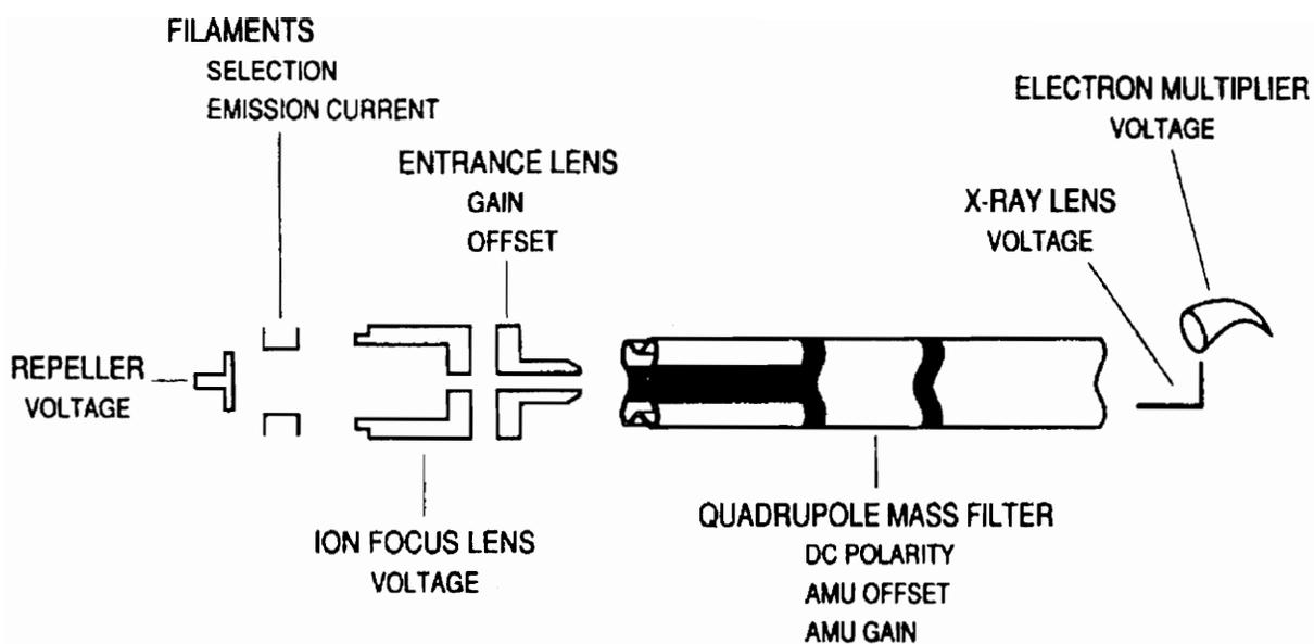
**FIGURE 5:** Parts Affected by Tuning<sup>(17)</sup>
