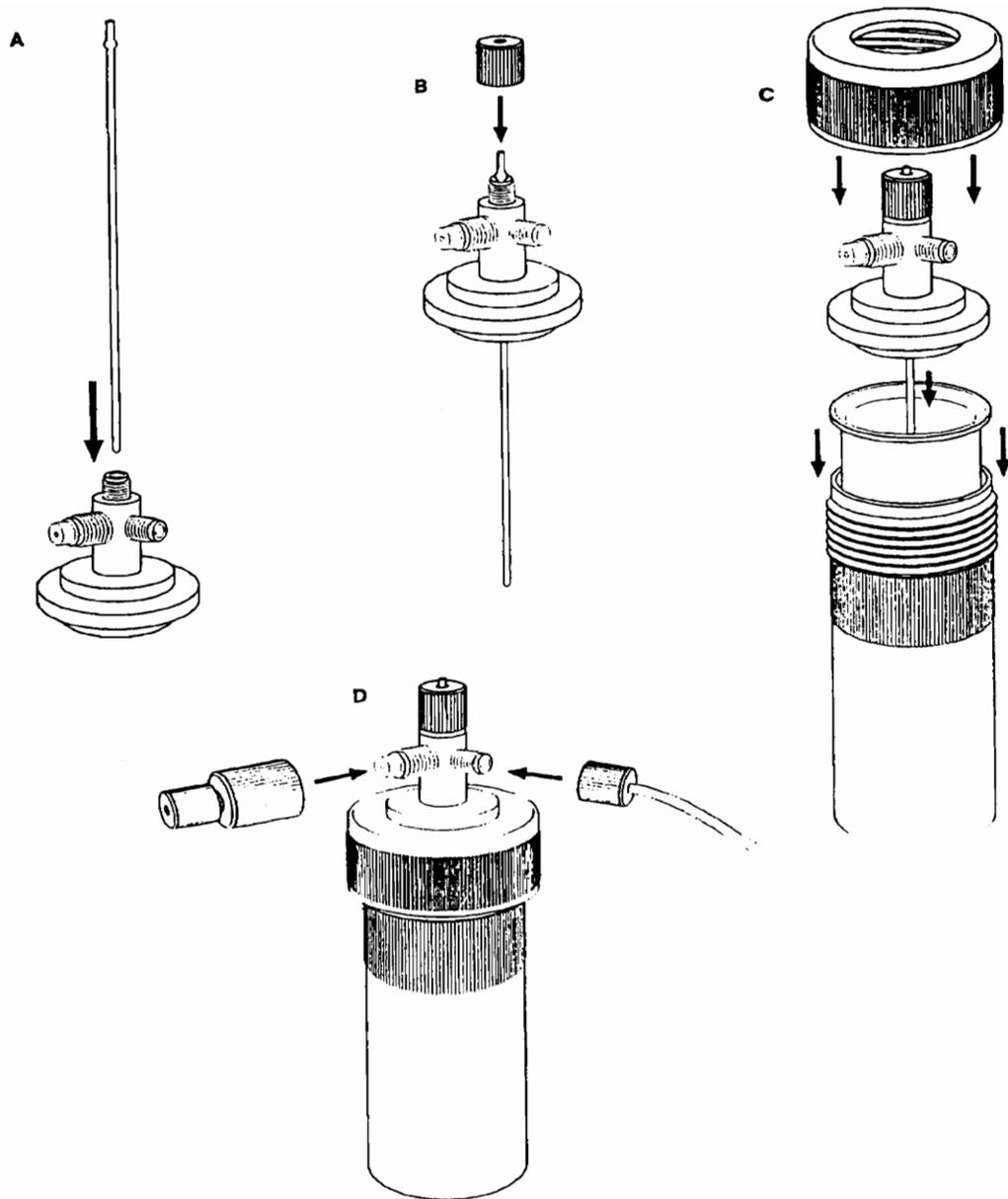
**FIGURE 8:** Assembly of Lined Extraction Vessel for Temperature and Pressure Control<sup>(18)</sup>
