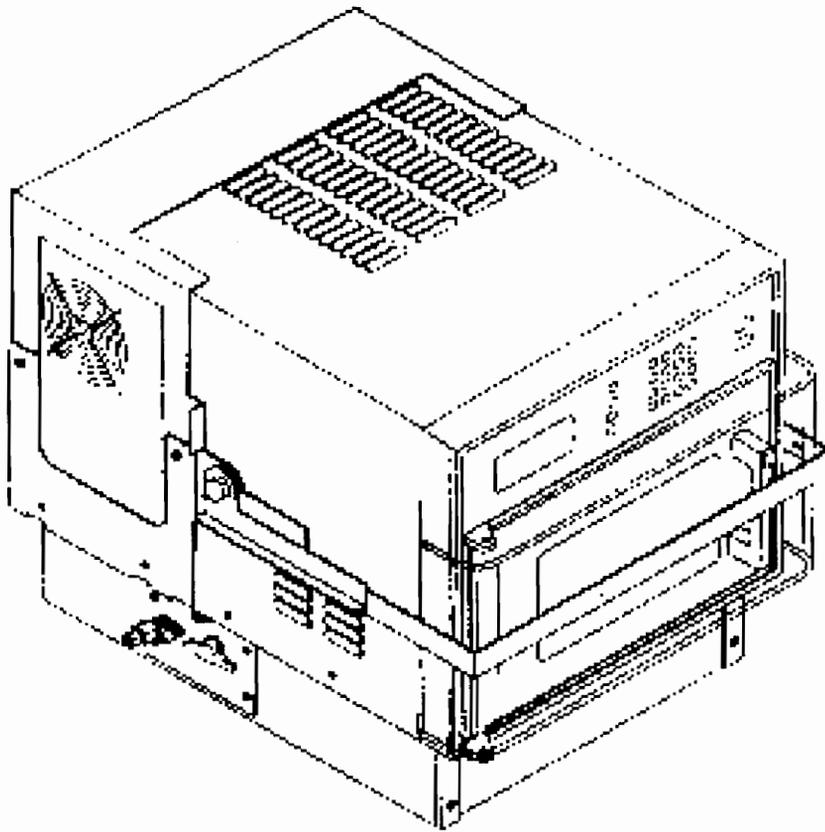
**FIGURE 6:** MES-1000 Microwave solvent extraction system<sup>(18)</sup>
