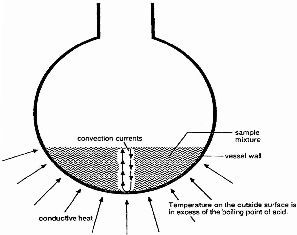
**FIGURE 1:** Diagram of sample heating by conduction<sup>(8)</sup>
