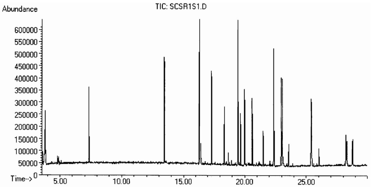
**FIGURE 24:** Typical chromatogram of a Chloroform Soxhlet Spike
