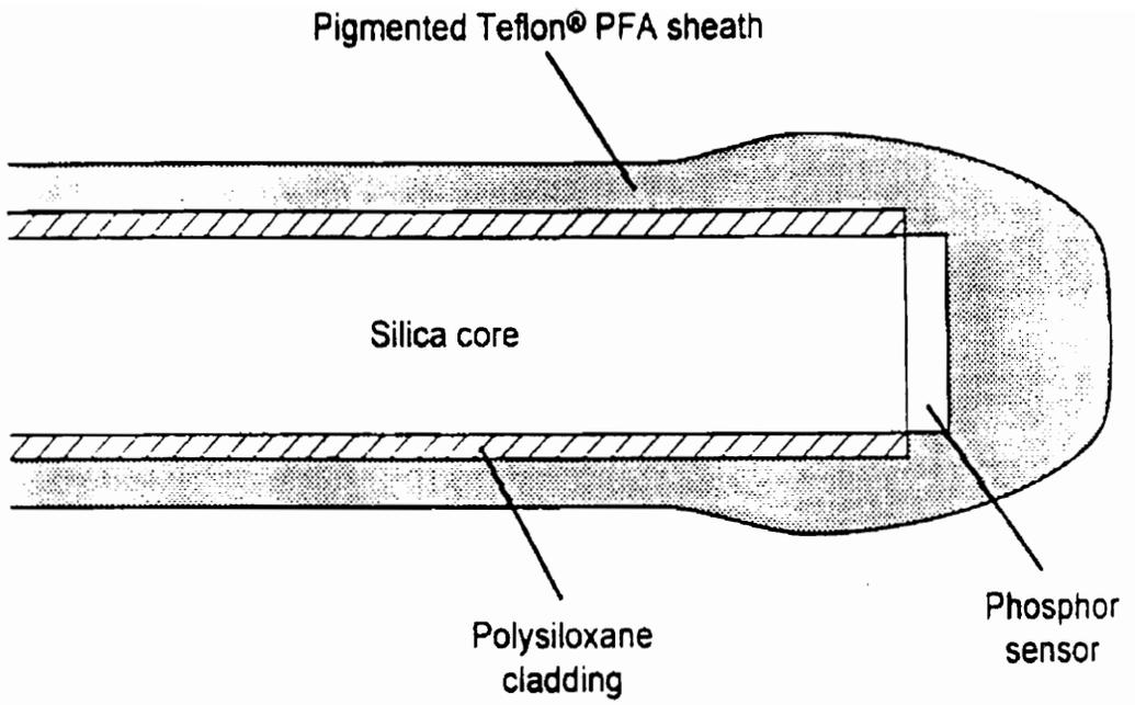
**FIGURE 9:** Fiber Optic Thermometry Probe<sup>(18)</sup>
