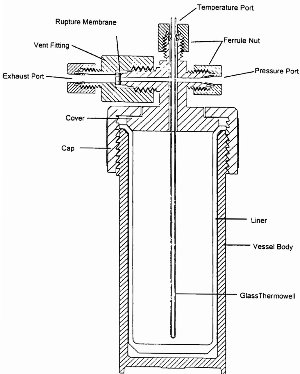
**FIGURE 7:** Lined Extraction Vessel for Temperature and Pressure Control<sup>(18)</sup>
