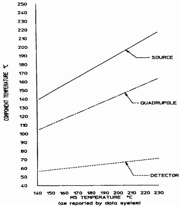
**FIGURE 4B:** Component Temperatures vs. MS Temperature<sup>(17)</sup>
