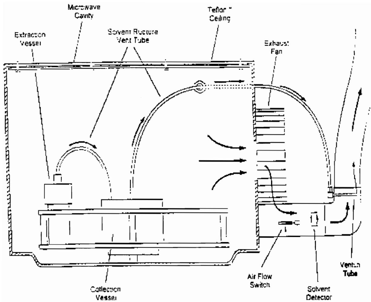
**FIGURE 12:** Safety Features of microwave solvent extraction system<sup>(10)</sup>
