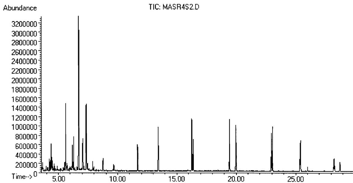
**FIGURE 25:** Typical chromatogram of an Acetone Microwave Spike
