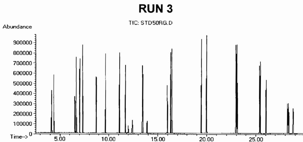
**FIGURE 19:** Triplicate Analyses of the 50 ng/ $\mu$ L Standard
