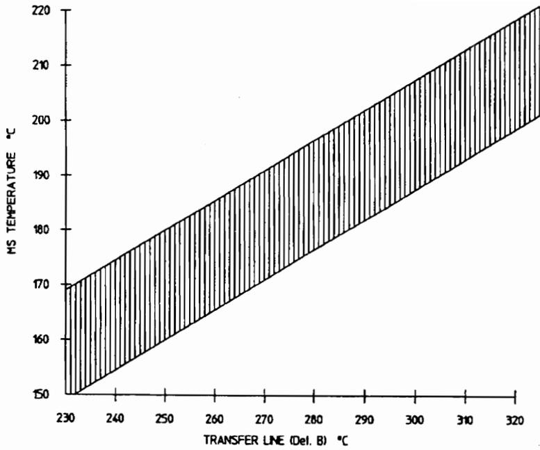
**FIGURE 4A:** MS Temperature vs. GC/MSD Interface Temperature<sup>(17)</sup>
