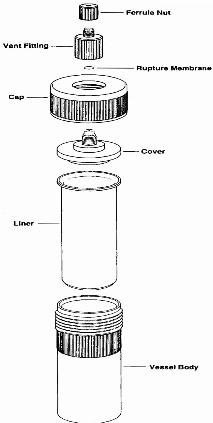
**FIGURE 11:** Lined Extraction Vessel (Exploded View)<sup>(18)</sup>
