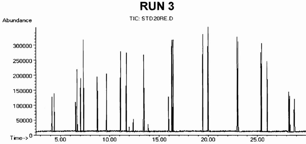
**FIGURE 18:** Triplicate Analyses of the 20 ng/ $\mu$ L Standard
