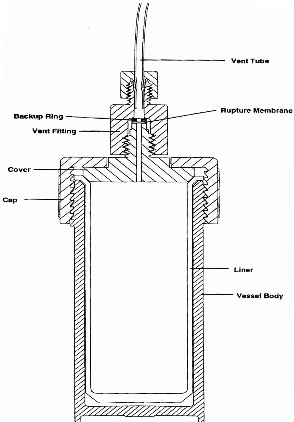
**FIGURE 10:** Lined Extraction Vessel<sup>(18)</sup>
