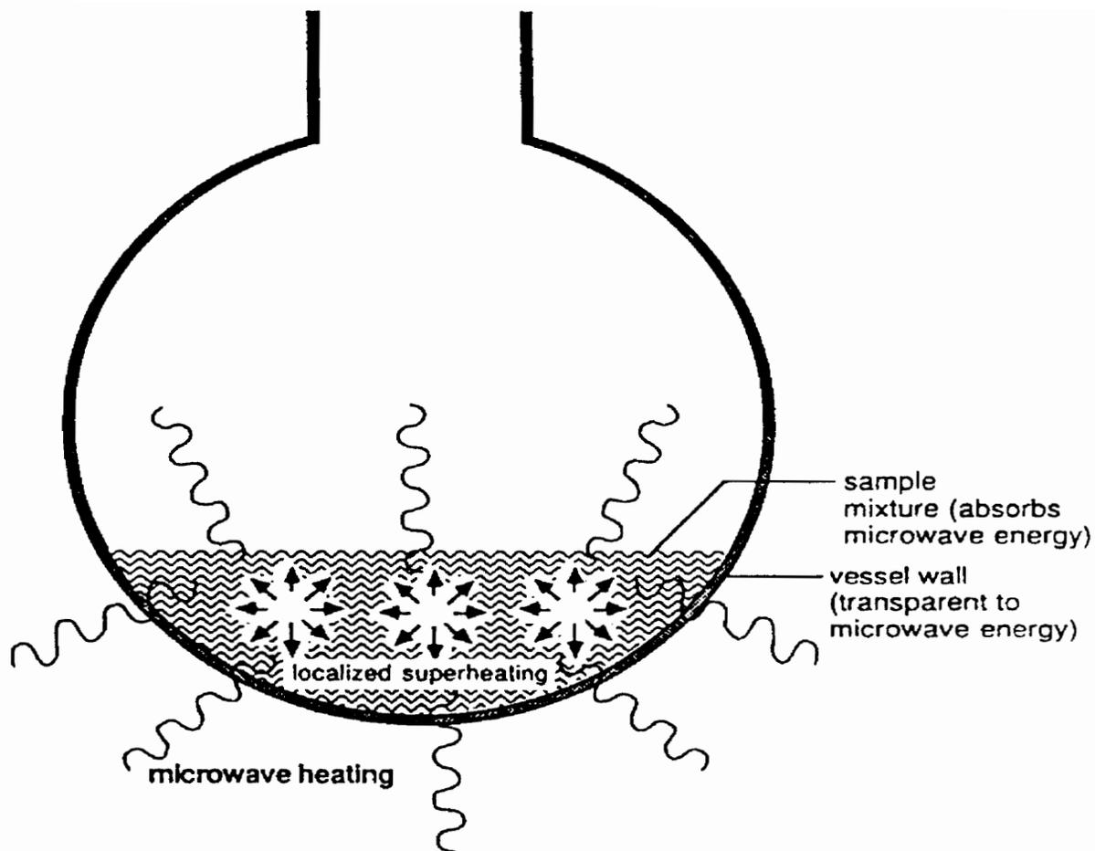
**FIGURE 2:** Schematic of sample heating by microwave energy<sup>(8)</sup>
