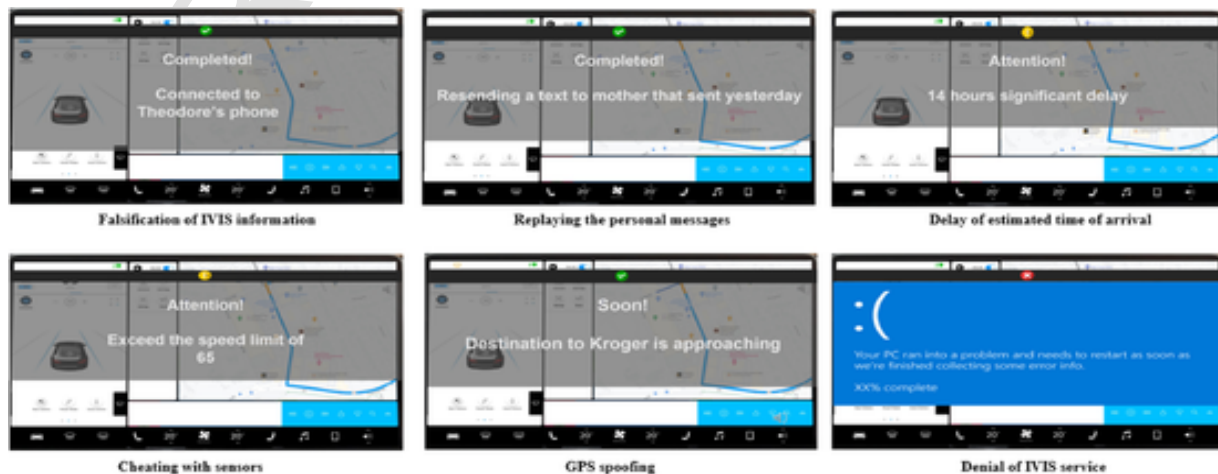
Fig. 3. Cyber-attacks alerts are displayed on the IVIS screen.
