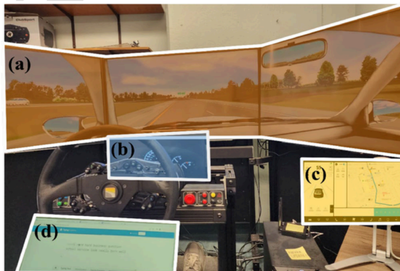
Fig. 1. Experimental setup with four AOIs (left). The four AOIs are on the left: (a) road, (b) dashboard, (c) IVIS screen, and (d) NDRT interface.
