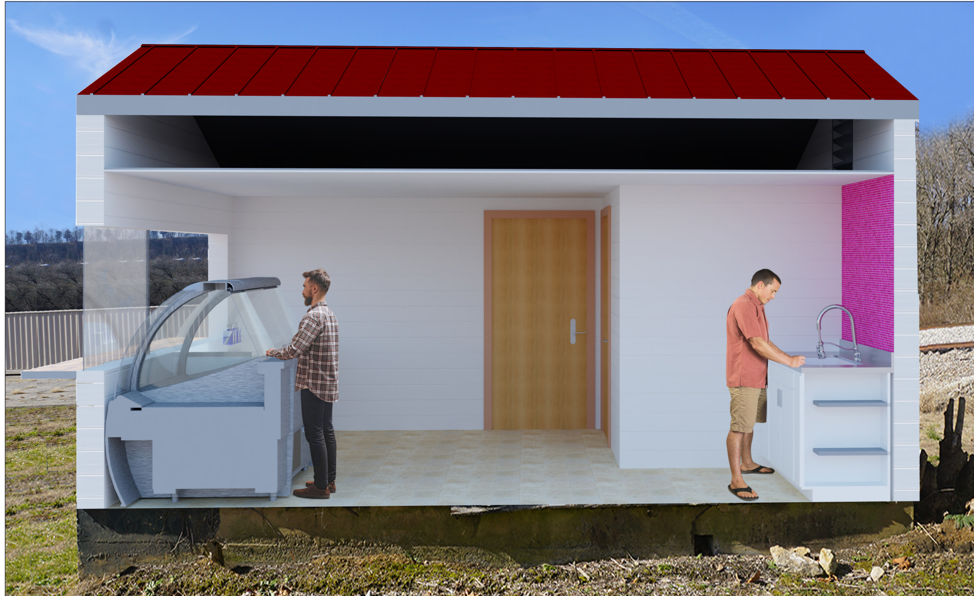
Section: Indoor Serving/Employee Area There is a toppings counter with two adjacent ice cream displays. There is also a cold storage space, sink, and undercounter refrigerators for cold topping storage.
