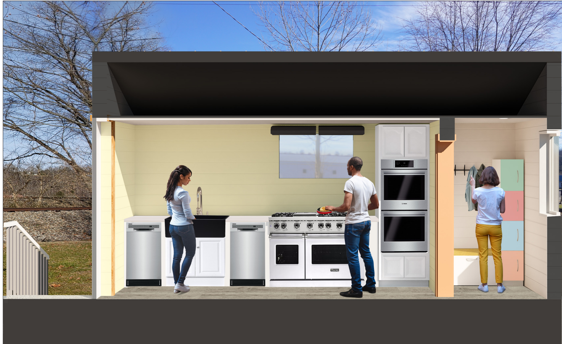
Perspective 2: Kitchen and Employee Personal Storage The kitchen is equipped with two dishwashers, a large sink, a cooktop and warming station, and two ovens. There is also cold storage and prep space. Employee personal storage is provided at the front of the building.
