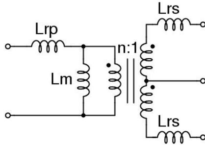
Figure 5.7 Magnetic components configuration from real transformer
