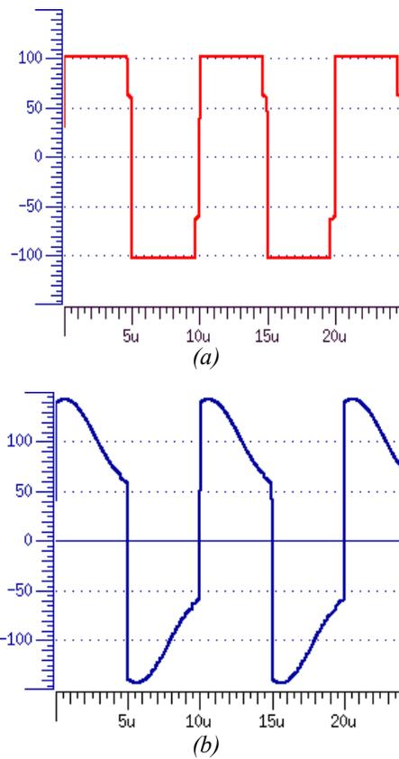
Figure 5.8 Voltage stress of output diodes D1 D2 (a): desired structure (b) real transformer
