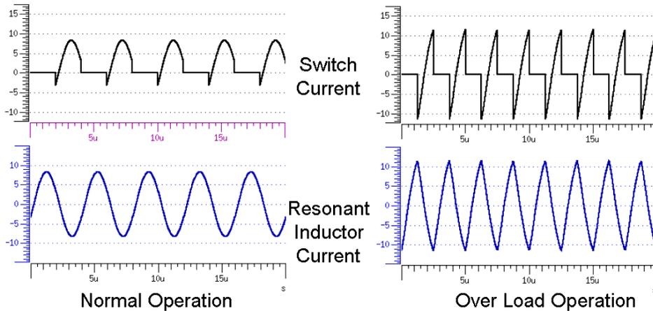
Figure 5.32 Problems with high switching frequency protection mode
