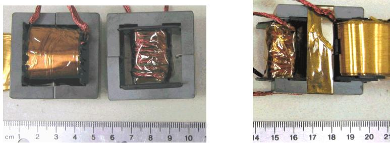
Figure 5.23 Magnetic size comparison of discrete and integrated magnetic
