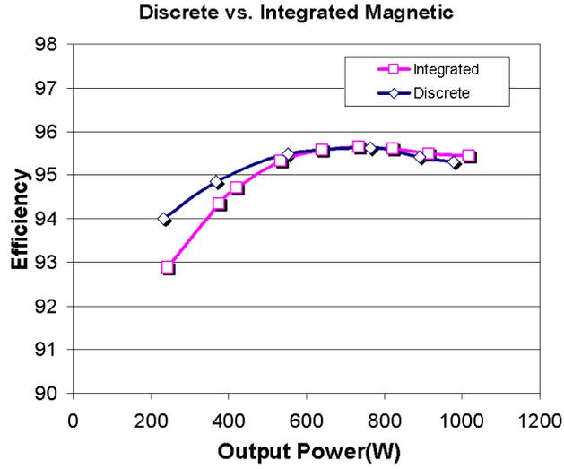
Figure 5.22 Efficiency comparison of integrated and discrete magnetic design for LLC converter
