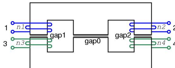
Figure 5.12 general magnetic structures for Integrated magnetic
