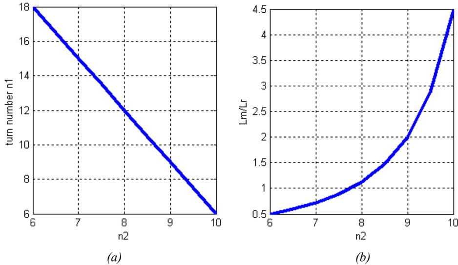
Figure 5.20 Design curves for integrated magnetic structure B for LLC converter
