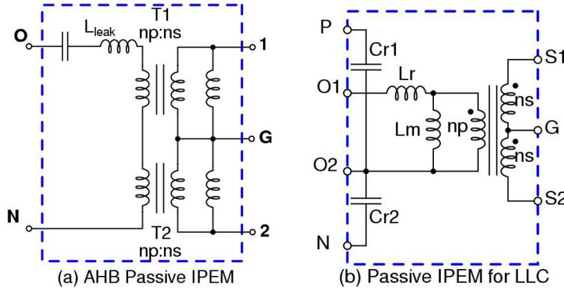
Figure 5.47 Schematics of passive IPEM for AHB and LLC r converter
