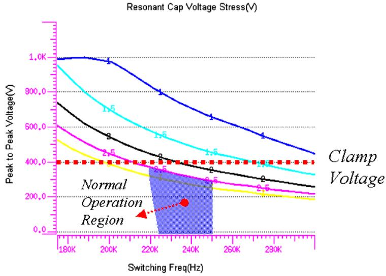
Figure 5.44 Design region of clamped LLC resonant converter
