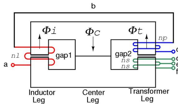
Figure 5.9 Integrated Magnetic Designs A
