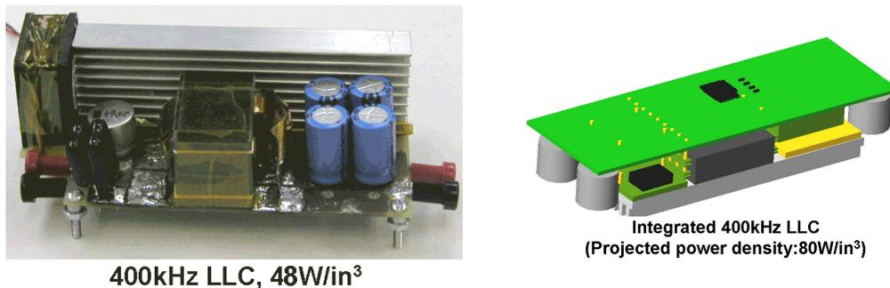
Figure 5.50 Power density of discrete LLC and projected integrated LLC
