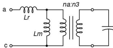
Figure 5.19 Equivalent-circuit for mode (a)
