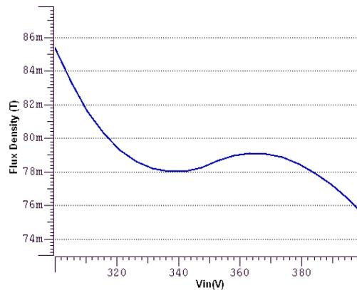
Figure 5.11 Center leg flux density for different input voltage
