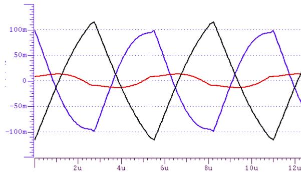
Figure 5.21 Flux density in each leg for integrated magnetic structure B
