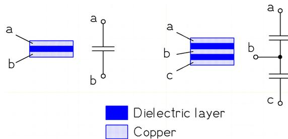
Figure 5.48 Capacitor integration for LLC resonant converter
