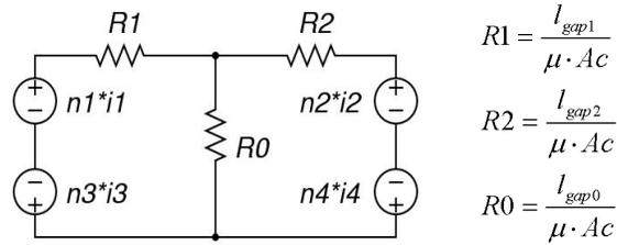
Figure 5.13 Reluctance model of general integrated magnetic structure
