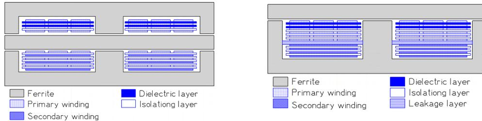
Figure 5.49 Two passive IPEM structures for LLC resonant converter
