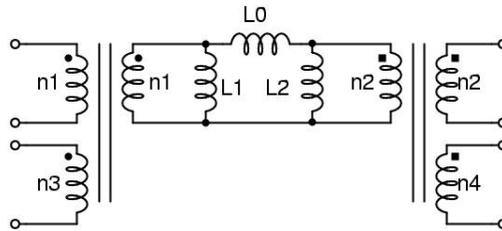
Figure 5.14 Circuit model of general integrated magnetic structure
