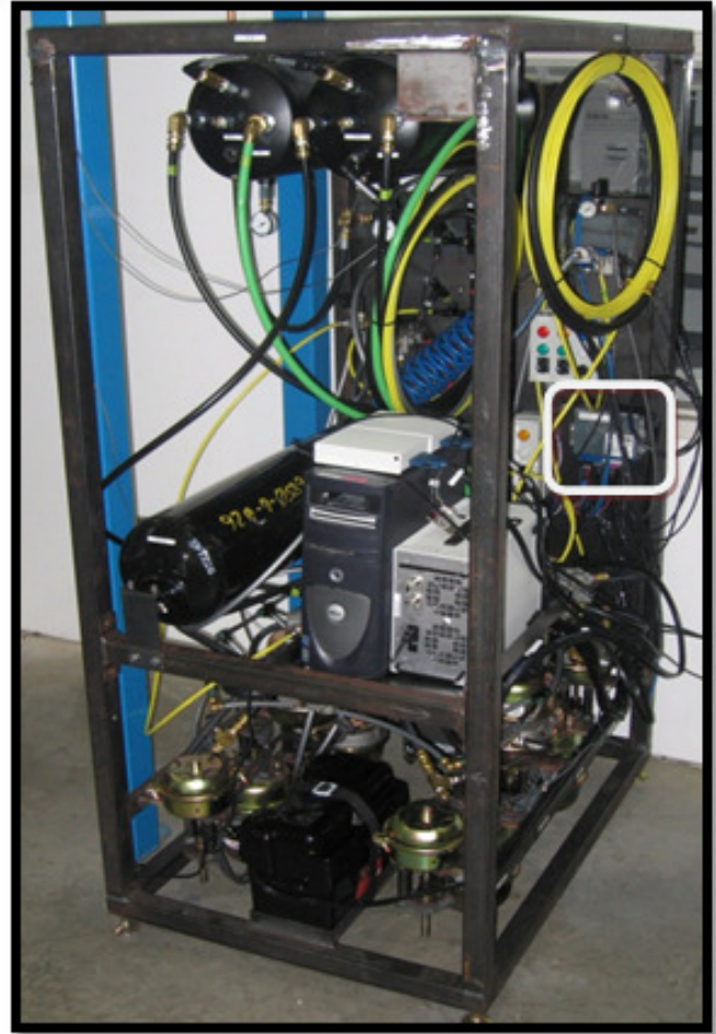
Figure 5: Front view of full braking system incorporated in the HiL system. The Bendix Electronic Stability Program is outlined in the white box. The gray computer on the left is the server and the off white computer on the right is the real-time unit. Below the computers are the brake chambers for both the tractor and the trailer.
