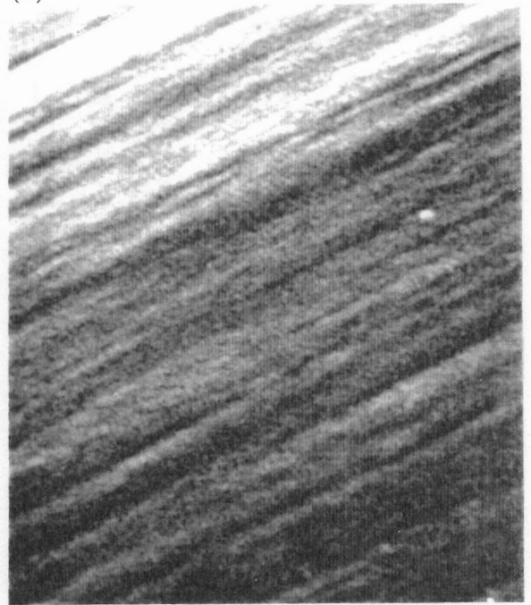
Figure 2.56. SEM photomicrographs of (a) "as received," (b) 15 sec. air plasma, (c) 15 sec. oxygen plasma, and (d) 1 min. ammonia plasma treated AS-4 carbon fibers at a magnification of 50,000X.
