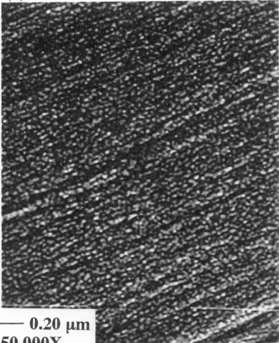
Figure 2.56. SEM photomicrographs of (a) "as received," (b) 15 sec. air plasma, (c) 15 sec. oxygen plasma, and (d) 1 min. ammonia plasma treated AS-4 carbon fibers at a magnification of 50,000X.
