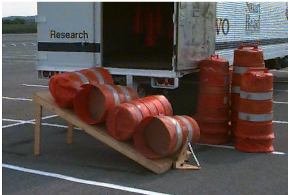
Figure 7. Ramp used to present obstacles.
