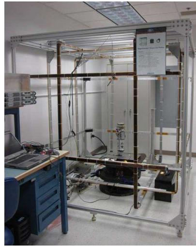
(b) SDL Helmholtz cage for magnetic field simulation [44]
