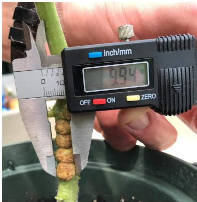
Figure 2-1. Measurement of tomato stem galls 42 days after inoculation with a digital caliper. Each gall diameter was measured at the widest point.
