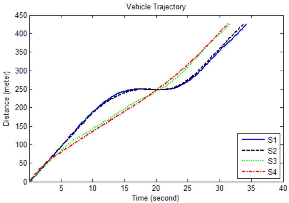
Figure 24: Example of vehicle speed profile and trajectory under red phase offset 20 seconds, downhill direction.
