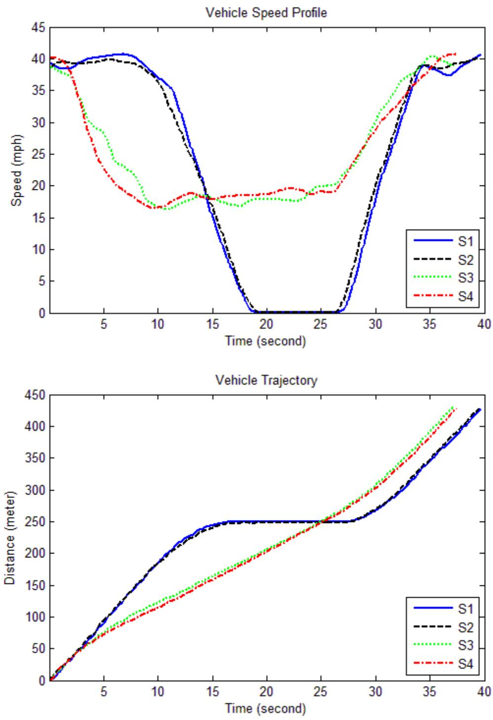
Figure 26: Example of vehicle speed profile and trajectory under red phase offset 25 seconds, uphill direction.
