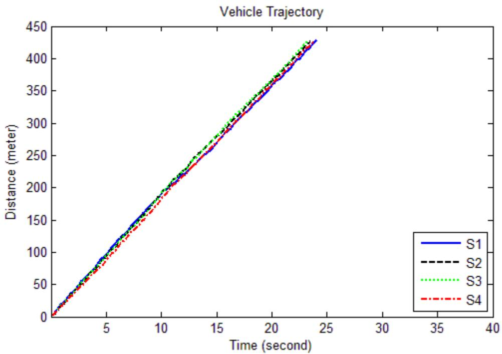
**Figure 13: Example of vehicle speed profile and trajectory under red phase offset 10 seconds, uphill direction.**
