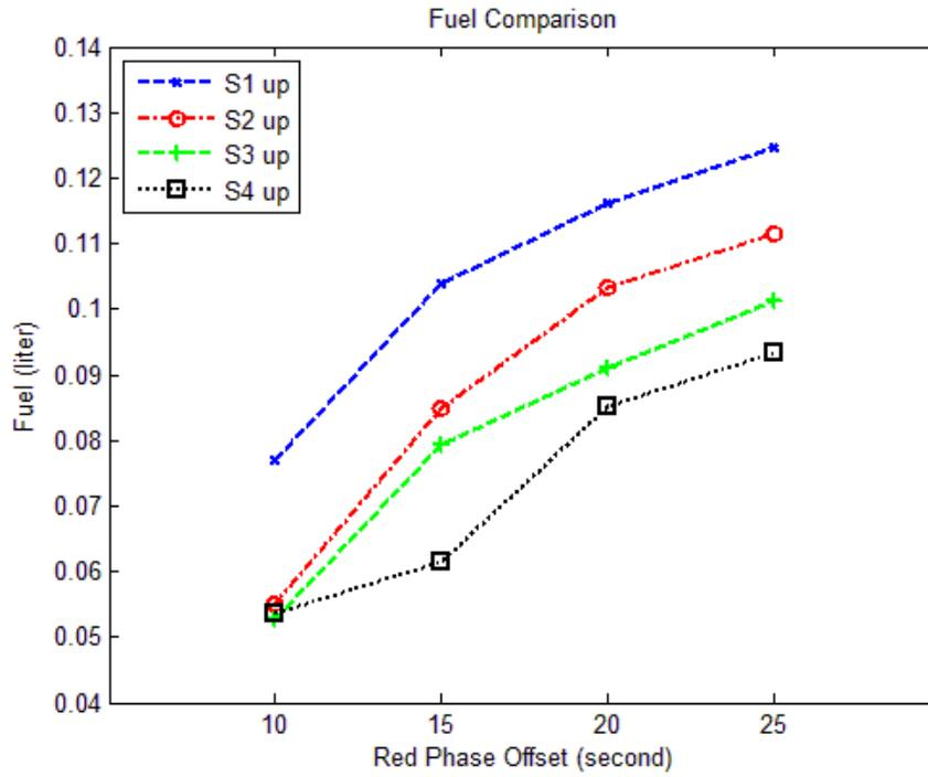
Figure 9: Comparison of fuel consumption for different scenarios for uphill direction.
