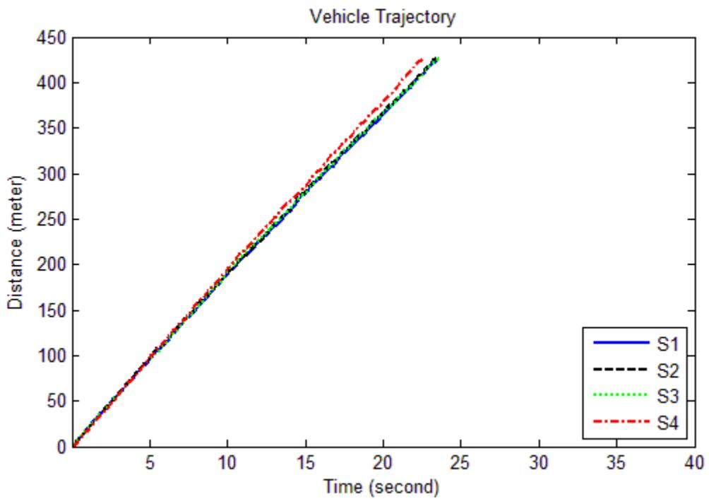
Figure 12: Example of vehicle speed profile and trajectory under red phase offset 10 seconds, downhill direction.
