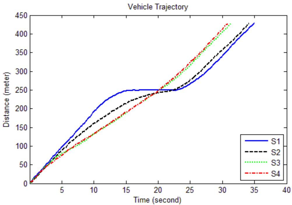
Figure 14: Example of vehicle speed profile and trajectory under red phase offset 20 seconds, uphill direction.
