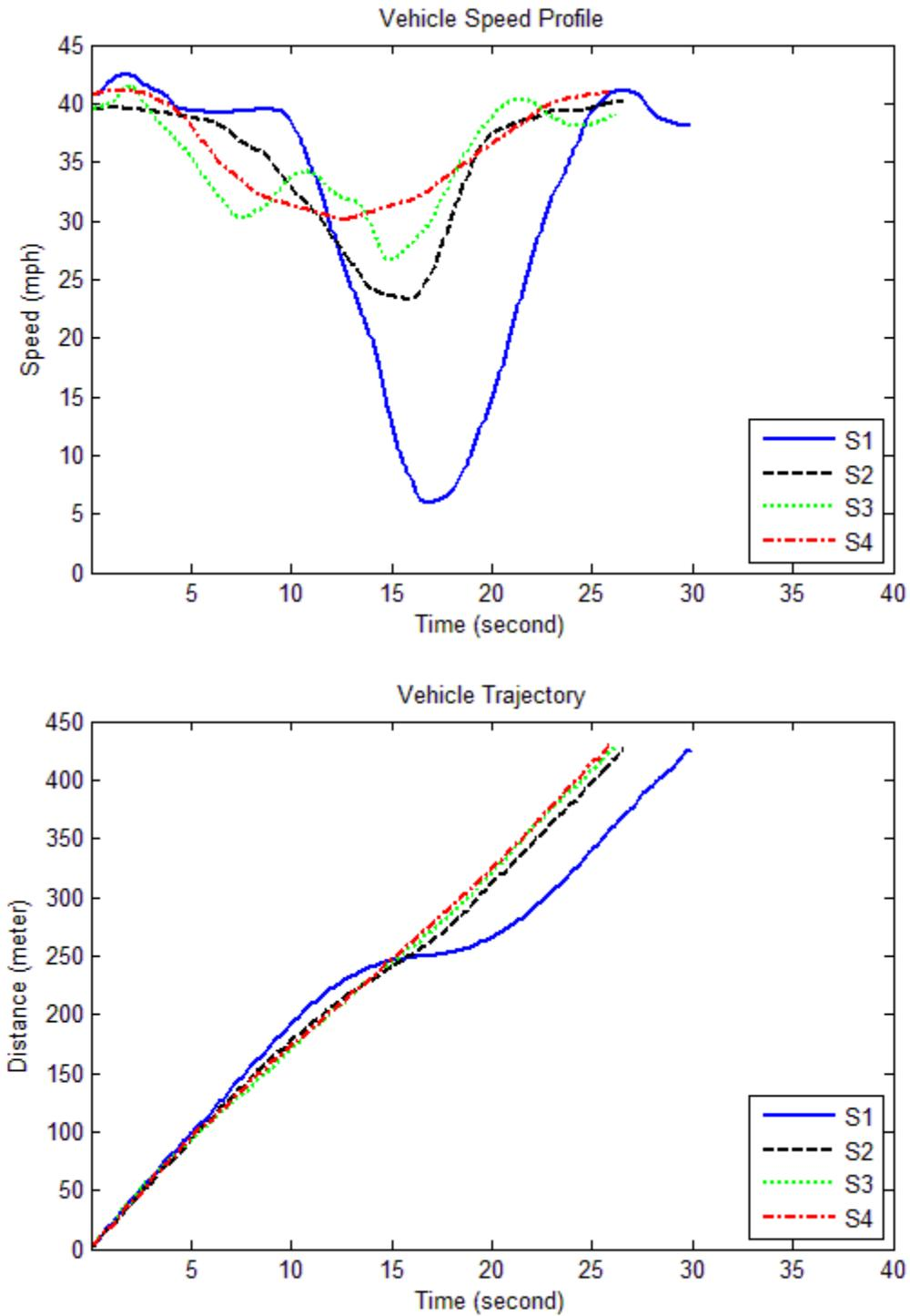
Figure 22: Example of vehicle speed profile and trajectory under red phase offset 15 seconds, downhill direction.
