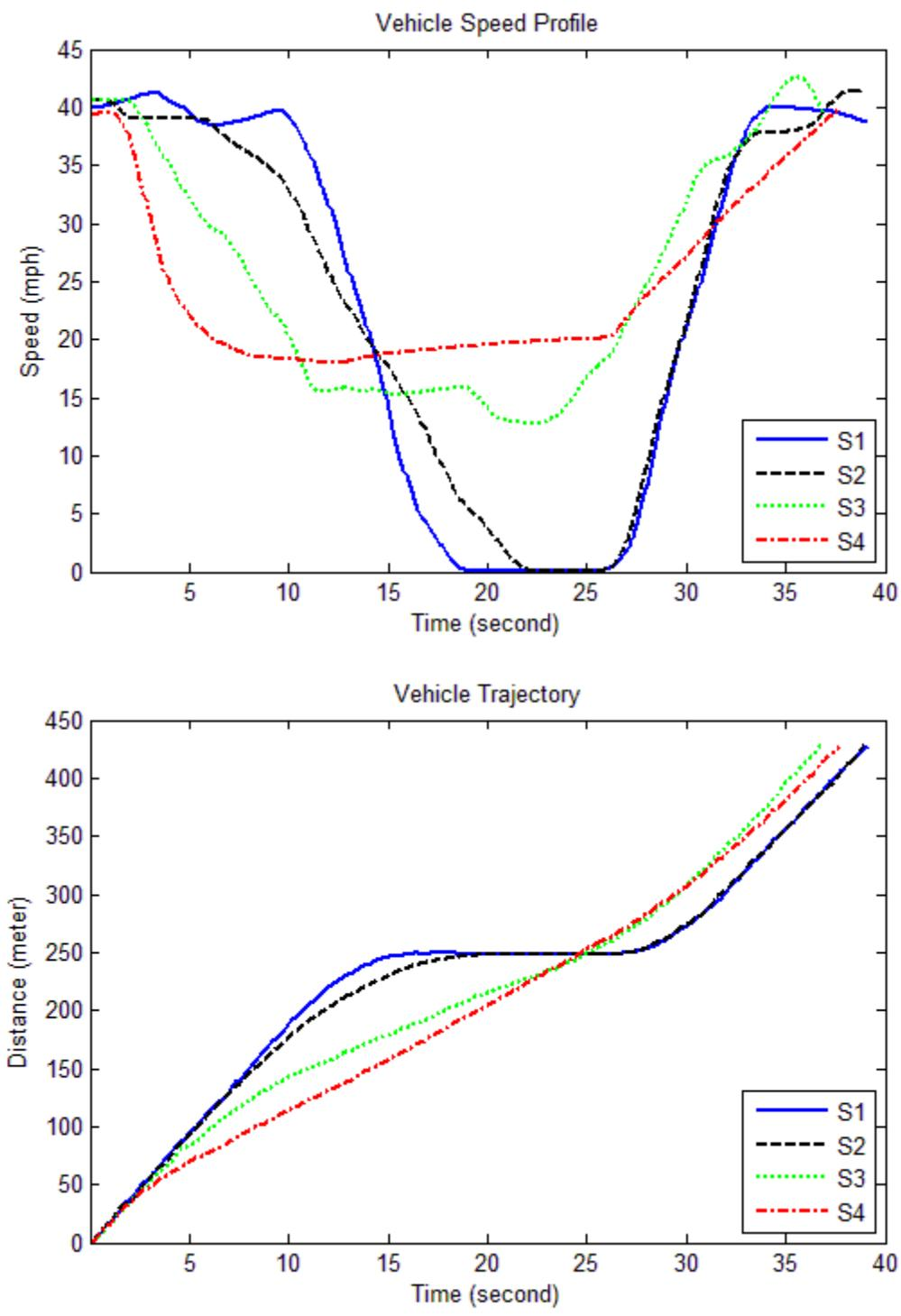
Figure 25: Example of vehicle speed profile and trajectory under red phase offset 25 seconds, downhill direction.
