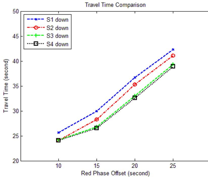
Figure 10: Comparison of travel time for different scenarios for downhill direction.
