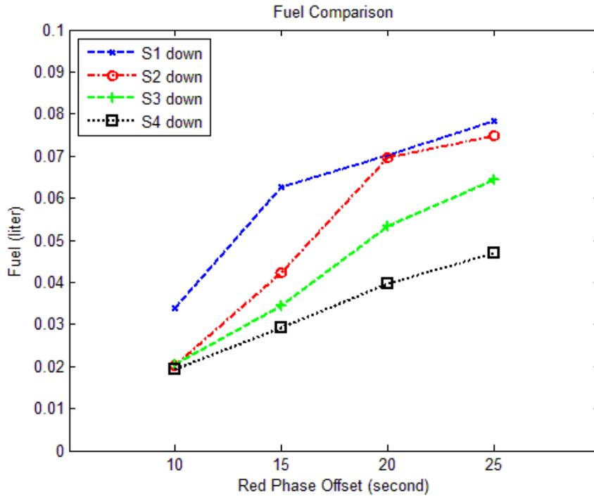
**Figure 8: Comparison of fuel consumption for different scenarios for downhill direction.**
