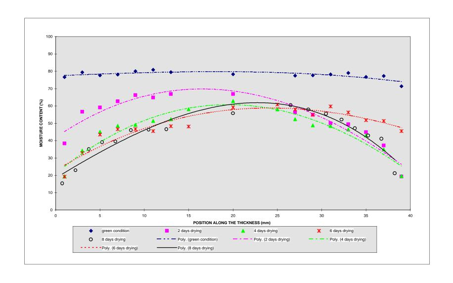
Figure 3.1. Moisture gradients measured on five different days by the Bandsaw slicing technique.
