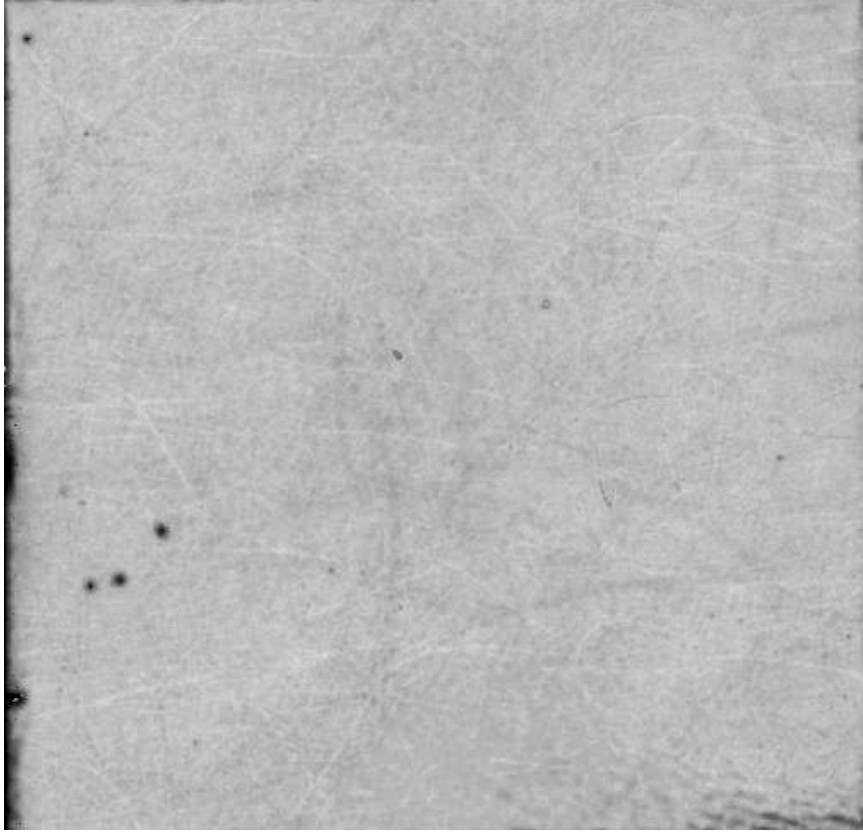
Figure 3.18 A C-scan image of Glass/PP plaque
