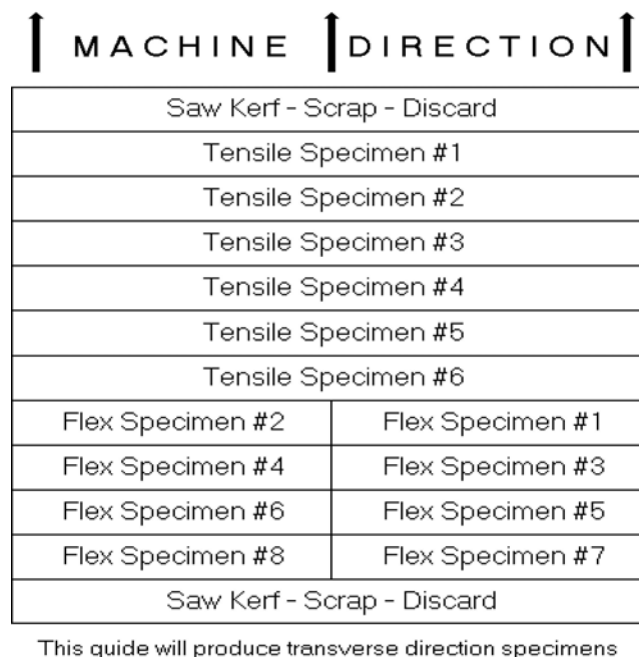
Figure 3.20 Test specimens cut in transverse direction
