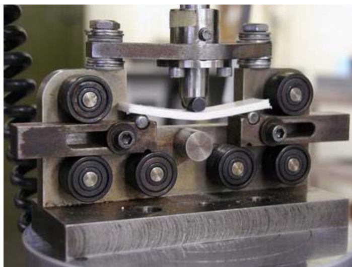
Figure 3.24 Three-point bending test
