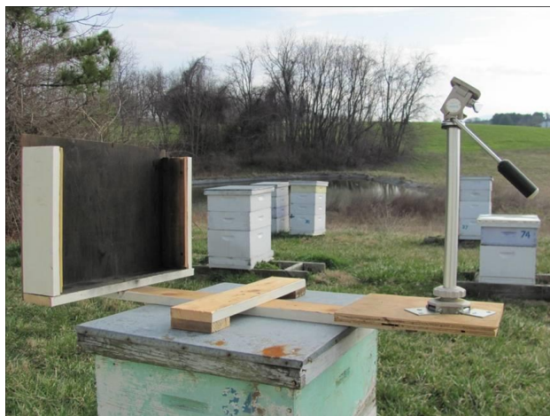
Fig. 3.1. Camera and brood frame holding device. On the left is the frame holder; on the right is the tripod for the camera.
