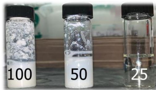
Figure 5. Comparison of water solubility of BDSA-MTPP/BDSA-Na/ODA poly(amic acid)s. As the indicated mol % of BDSA-MTPP decreases, the solubility of the PAA increases. At 25 mol% BDSA-MTPP, the PAA is fully soluble.
