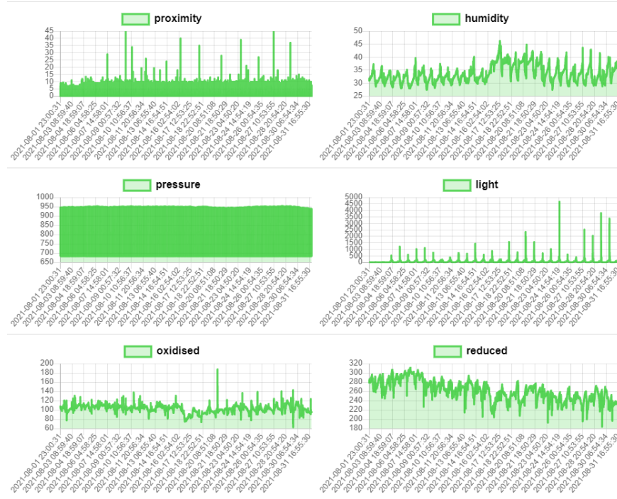
Figure 3.14: Visualization of collected data from all sensors of a deployed sensing node.
