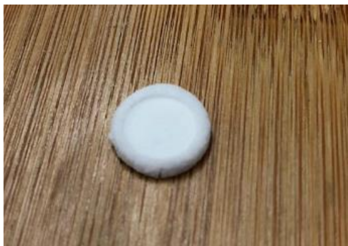
Figure 13, NF lactose monohydrate impalpable 312 powder combined with the 30wt% of corn starch and 20wt% of powdered sugar to printed with 40K PVP and DI water binder. Compression strength at different drying time
