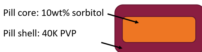
Figure 22. Schematic illustration of the pills printed with multi-binder
