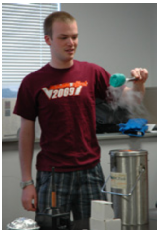
Kyle Novak (class of '12) explains the thermal expansion of air using liquid nitrogen and a balloon
