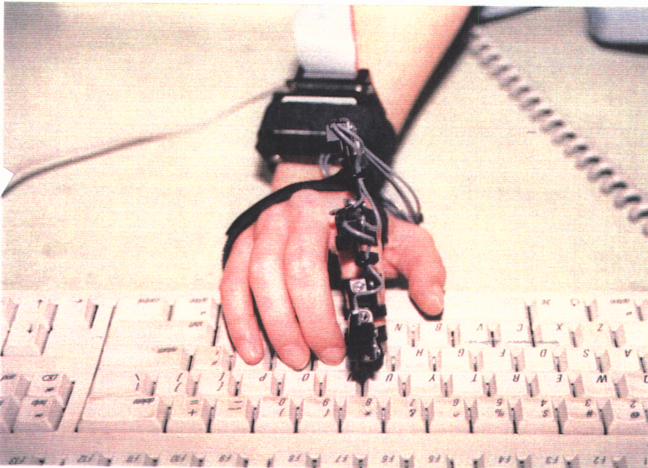
Figure 3.2 Modified DHM exoskeleton.
