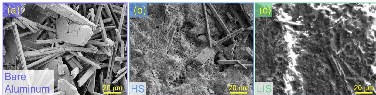
Figure 7.9. SEM image of aluminum-based surfaces after 96 h calcium dynamic fouling test at 200 rpm and room temperature. (a) Bare aluminum surface; (b) aluminum hydrophobic surface (HS); (c) aluminum lubricant infused surface (LIS).
