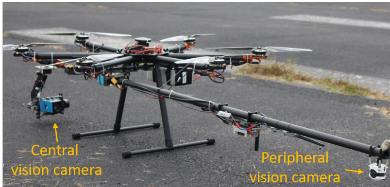
Figure 3.2: Peripheral-central vision (PCV) system setup.
