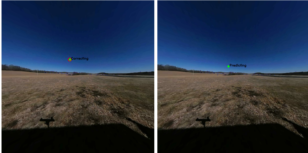
Figure 3.7: Example results of the optical flow detection with Kalman filter (red circle on the left indicates a moving object detected by optical flow. The Kalman filter corrects its estimation (a green dot) based on the detection. There is no optical flow detection on the right, the Kalman filter predicts its estimation based on the estimated pixel position and velocity.)
