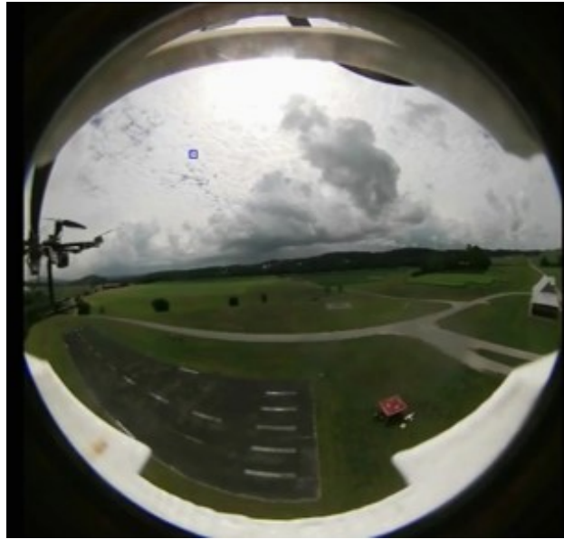
Figure 7.1: Lens distortion of a fisheye lens
