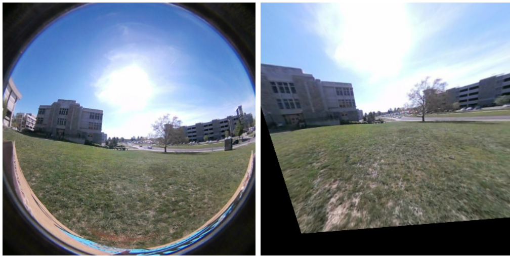
Figure 3.5: Peripheral vision image before (left) and after (right) undistortion and stabilization.
