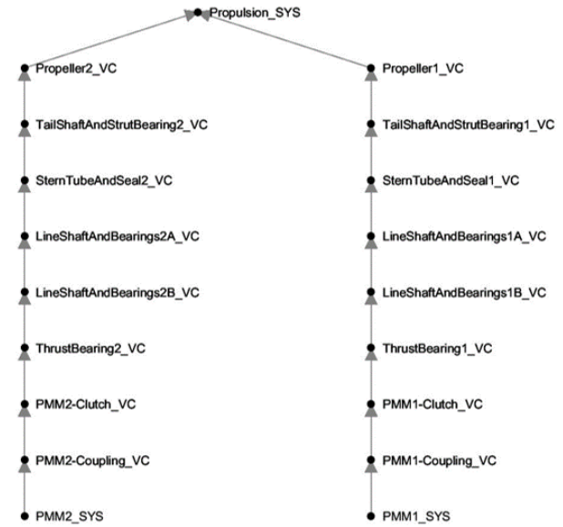
Figure 15. Mechanical (Propulsion) Subsystem (MECH)
