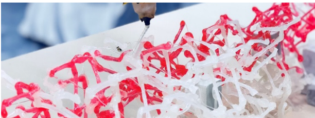
Figure 2: Spatial 3D printing of a lattice with multiple materials and differentiated polyhedral arrangements
