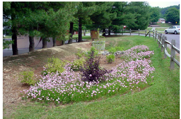
Rain gardens, such as this one in Blacksburg, VA, slow the flow of water and use it for the plants within.
