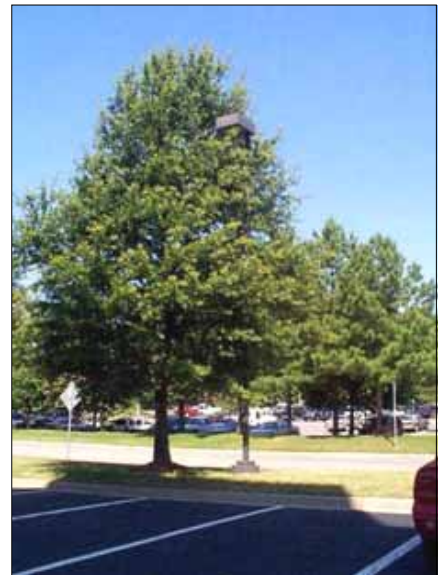
Separate trees from light poles for effective lighting in a parking lot. In this example in Chesterfield County, VA, the light is only illuminating the tree canopy.
