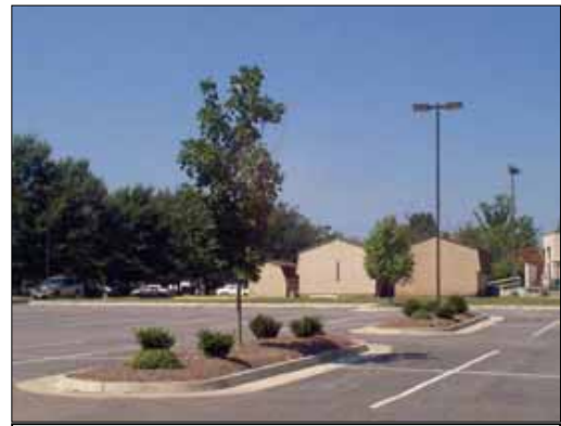
Alternate landscape and light islands within parking areas to prevent trees from growing up into the light fixtures. The above fixture is an example of a shoebox light fixture found in Chesterfield County, VA.
