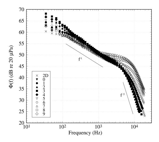
**Figure 52.** Spectral power density of p ( $Re_{\theta} = 23400$  (2-D); 23200 (3-D)). The numbers in the legend denote the measurement station.
