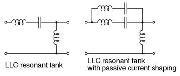
Figure 7.1 LLC resonant tank and LLC resonant tank with passive current shaping
