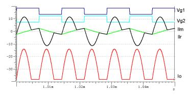
Figure 7.2 Simulation waveform of LLC resonant converter
