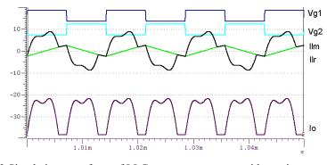
Figure 7.3 Simulation waveform of LLC resonant converter with passive current shaping
