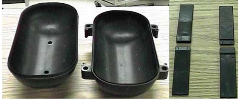
Figure 6-9: Picture of TNG joint used on an elliptical pressure vessel and a Nylon TNG test coupon.
