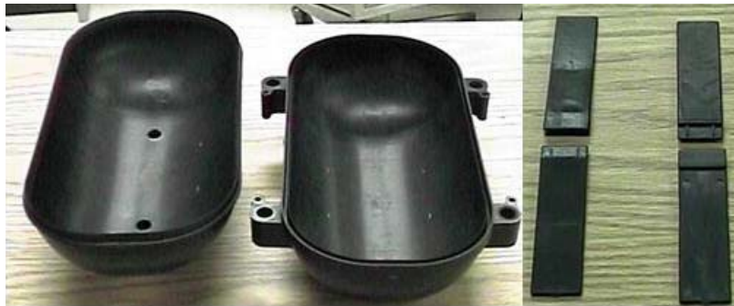
Figure 1-1: Two pictures of “Non-Standard”, but typical, joint configurations. Shown here, without adhesive applied, a flanged lip on a pressure vessel (left) and a TNG test coupon.
