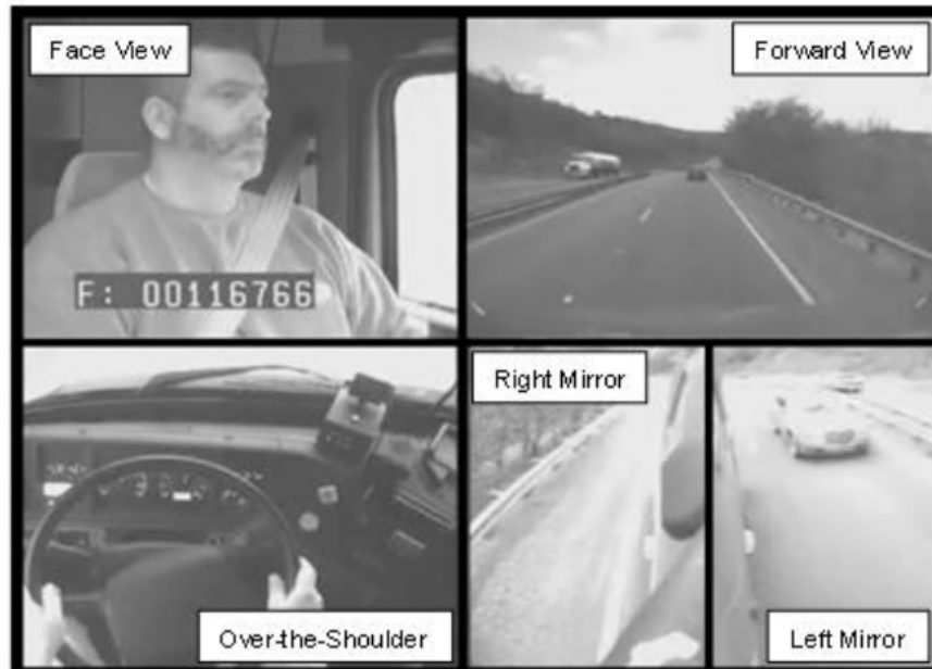
Figure 1.1: The Commercial Truck Driver NDS: Photo for five views from the installed video cameras (Blanco et al., 2011).
