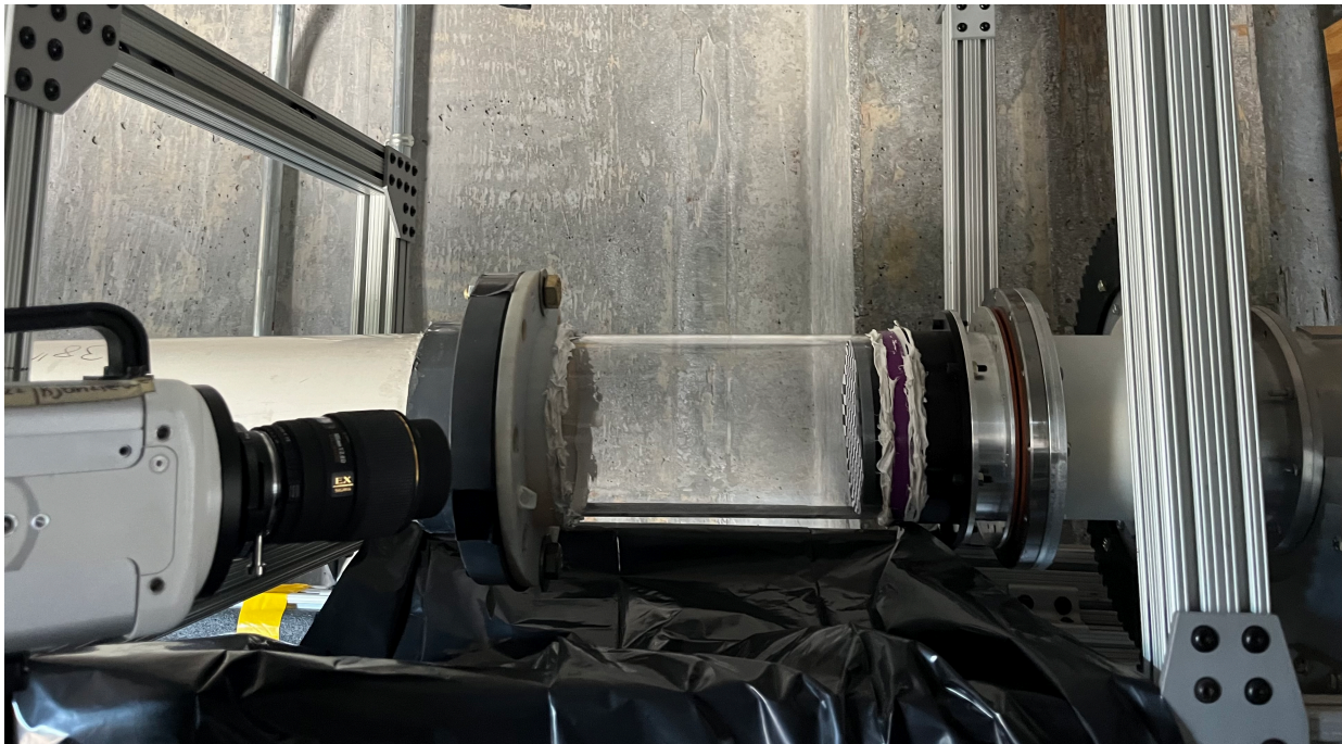
Figure 4.6: Image of the test section for the flow visualization experiment
