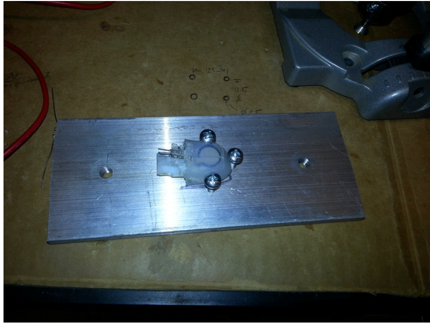
Figure 2-11: Aluminum plate with bolts to hold sensor sample in place.
