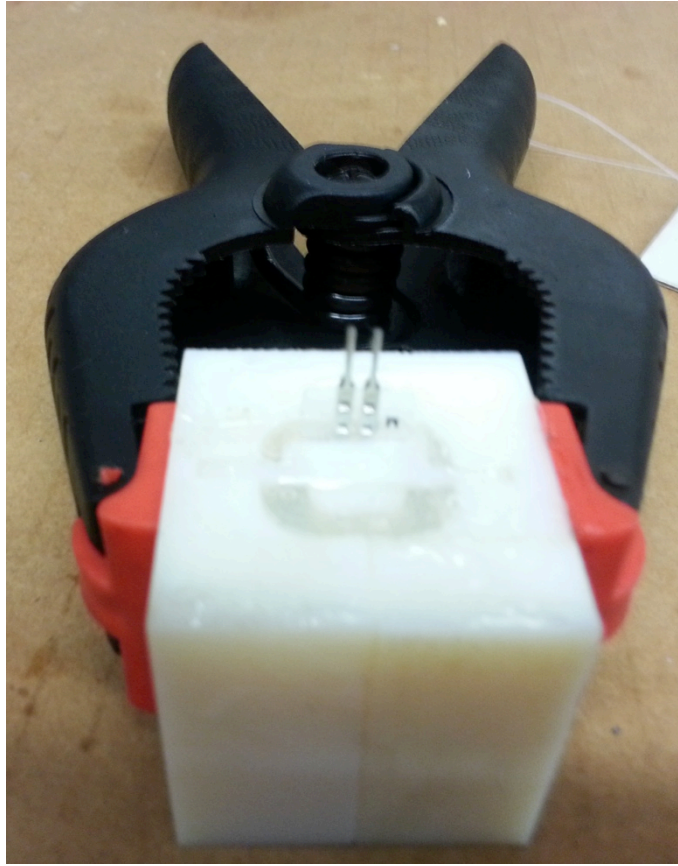
Figure A- 5: Full mold assembly clamped to cure.
