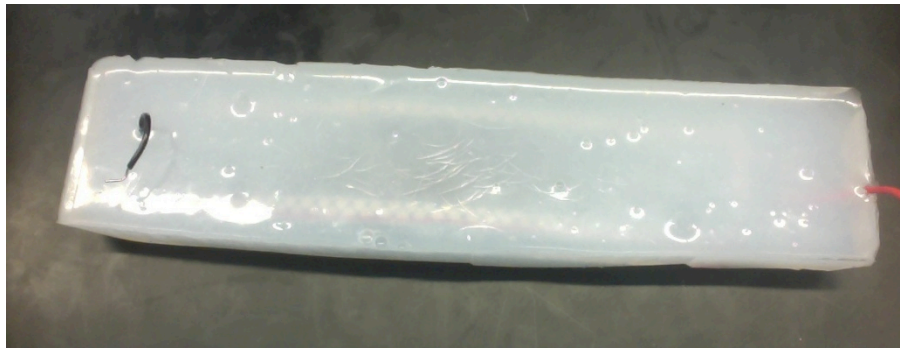
Figure 2-4: 6 inch fabric based sensor embedded in silicone.
