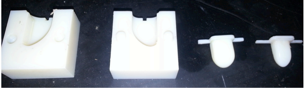
Figure A- 1: Negative molds(left) with .75 scale and .5 scale positive mold.
