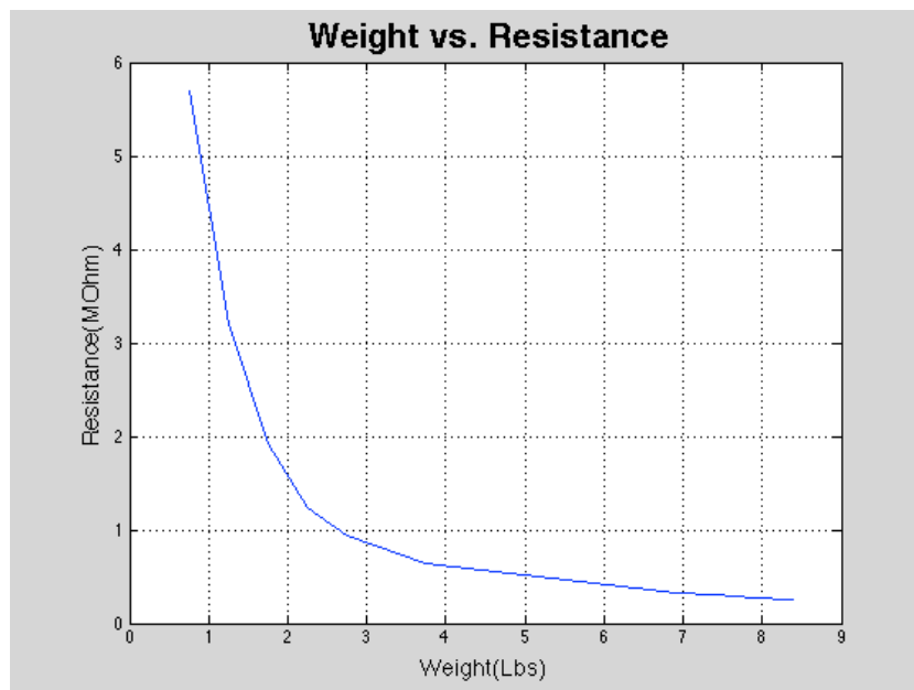
Figure 2-13: Plot of sensor response due to weight in terms of resistance
