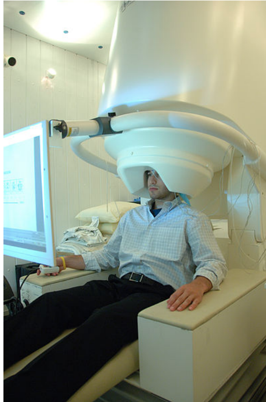
Figure 4-3: A subject using a MEG interface. Note the large device size and cooling necessary to use this method. National Institute of Mental Health. (2009).
