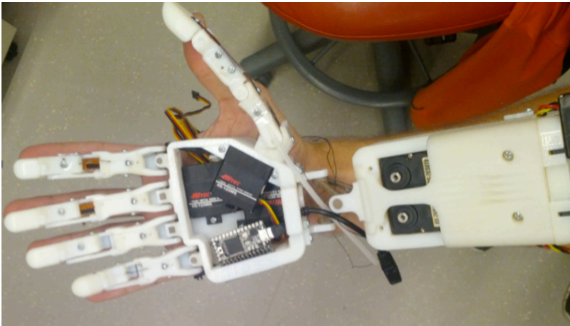
Figure 1-1: The Dexterous Anthropomorphic Sensing Hybrid(DASH) hand, shown in comparison with an adult male hand.
