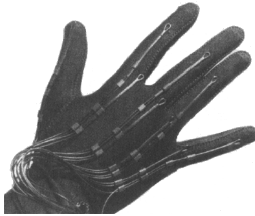
Figure 1-2: Sayre glove, with 10 degrees of freedom tracked using fiberoptic cables.
