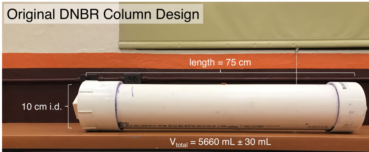
Figure 10 The original column design, which was modified for this experiment. Note that these columns were originally oriented vertically.
