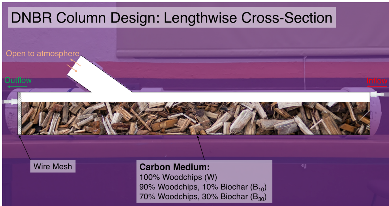
Figure 12 Lengthwise cross-section visual of an individual DNBR column, with flow from right to left. The wire mesh was added as a means to prevent media, particularly biochar, from washing out of the columns.
