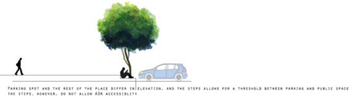
PARKING SPOT AND THE REST OF THE PLACE DIFFER IN ELEVATION, AND THE STEPS ALLOW FOR A THRESHOLD BETWEEN PARKING AND PUBLIC SPACE THE STEPS, HOWEVER, DO NOT ALLOW ADA ACCESSIBILITY
