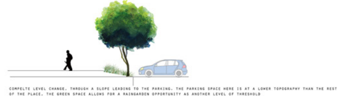
COMPLETE LEVEL CHANGE, THROUGH A SLOPE LEADING TO THE PARKING, THE PARKING SPACE HERE IS AT A LOWER TOPOGRAPHY THAN THE REST OF THE PLACE, THE GREEN SPACE ALLOWS FOR A RAINGARDEN OPPORTUNITY AS ANOTHER LEVEL OF THRESHOLD
