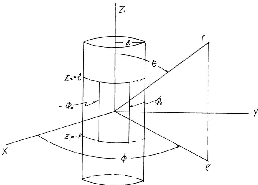
Fig. (4) Radiation from a transverse rectangular slot in a circular cylinder
