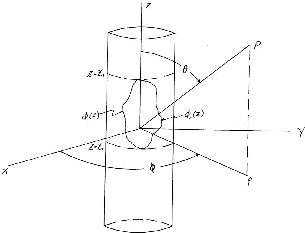
Fig. (3) Slotted cylinder antenna with infinite length
