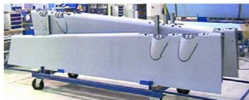
Figure 5: Internal and external ailerons (A340)
