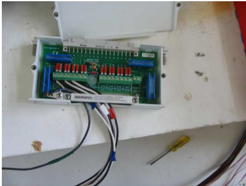
Fig 3.15 – SCXI-1327 Terminal Block
