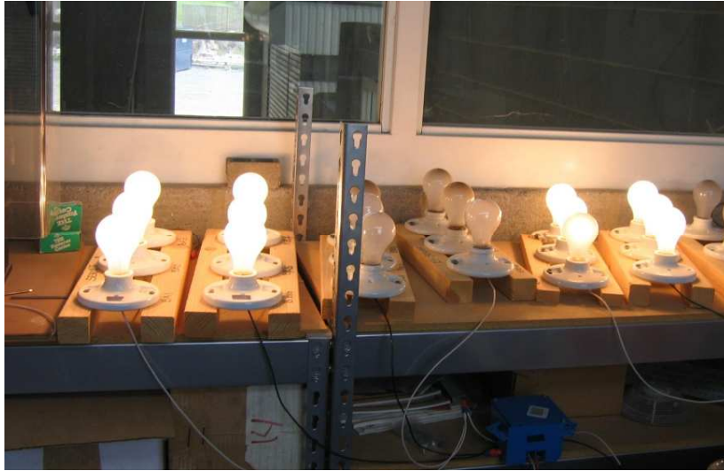
Fig 3.12 – DC light bulbs used as load
