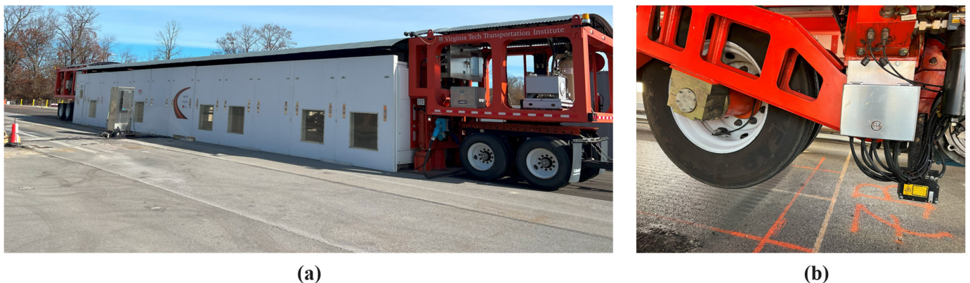
Figure 1. Photographs Taken of (a) Dynatest Mark VI Heavy Vehicle Simulator; (b) Laser Profiler Mounted on HVS Carriage.
