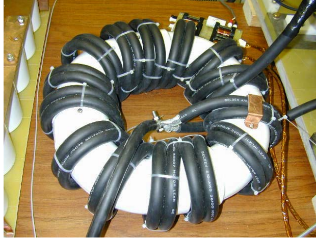
Figure 3-9. The air-core snubber inductor prototype.
