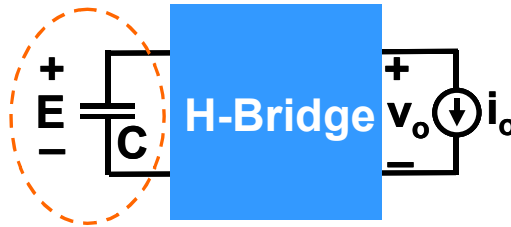
Figure 3-26. DC capacitor utilized in an H-bridge converter.
