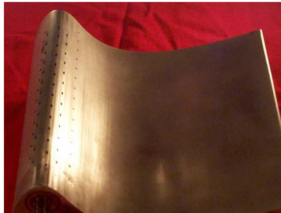
Figure 6.9: Photograph of the showerhead film cooling scheme
