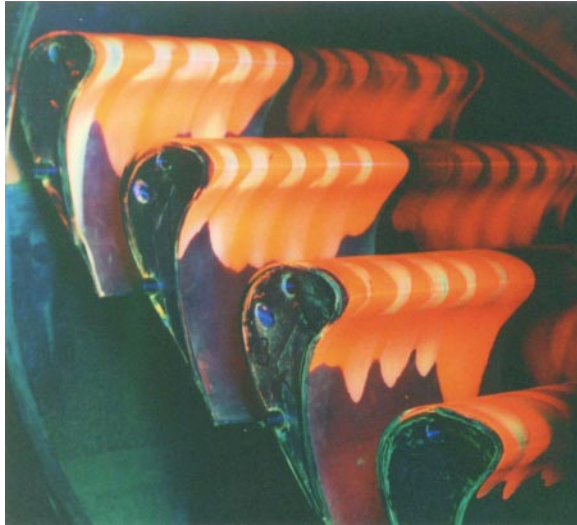
Figure 6.14: Oil flow visualization showing the positioning of the stagnation point on the blades.
