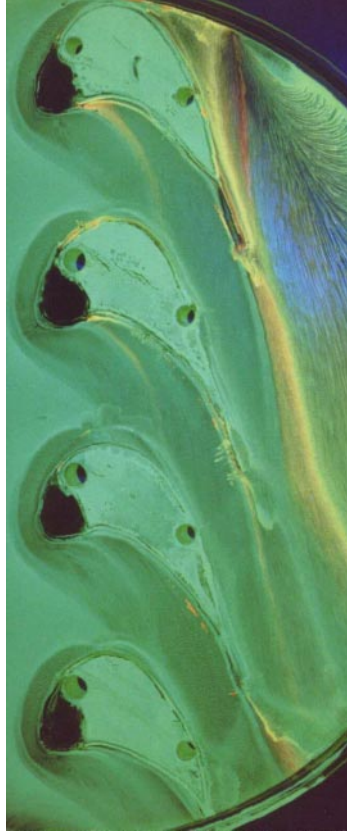
Figure 6.11: Oil flow visualization of the endwall
