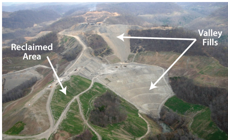
FIGURE 6.4 Mountaintop mining with associated valley fills. Note the inclusion of areas with AOCs, VFs, and reclamation efforts. SOURCE: McAtee, 2007.
