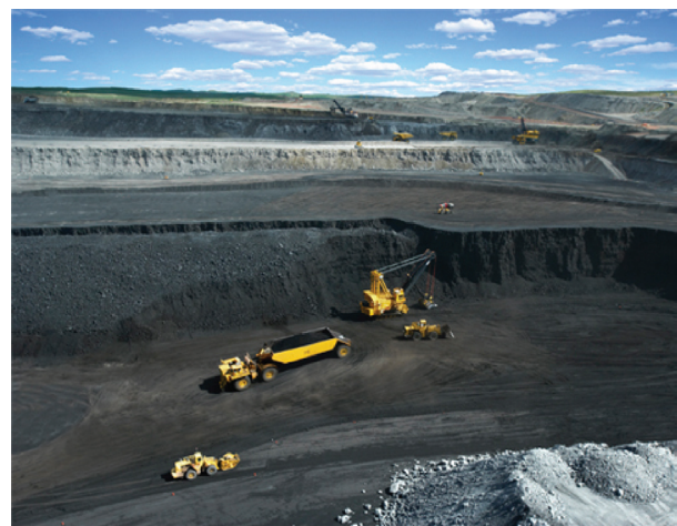
FIGURE 3.10 Powder River Basin surface coal mine. Notice the coal loading in the foreground, overburden removal in the background, and spoil dumped in the area where coal has been removed in the lower right hand corner. SOURCE: Peabody, http://www.peabodyenergy.com/Operations/coaloperations-PowderRiver.asp .
