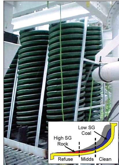
FIGURE 4.12 Bank of spirals used to separate fine coal and rock.
