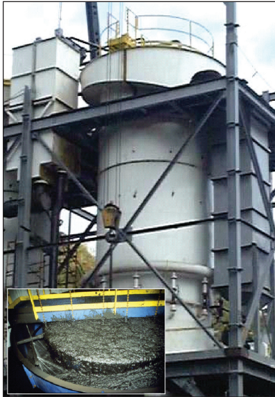
FIGURE 4.14 Column-type flotation cell used to clean ultrafine coal.
