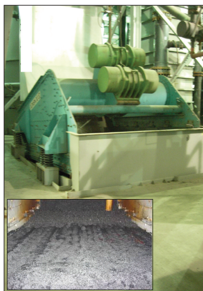
FIGURE 4.6 High-frequency screen used for dewatering of fine rock.
