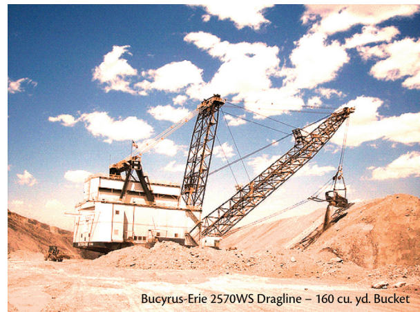
FIGURE 3.7 Example of a dragline operation. SOURCE: Bucyrus-Erie.
