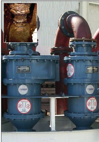
FIGURE 4.11 Bank of twin water-only cyclones used to separate fine coal and rock.
