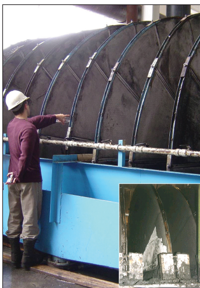
FIGURE 4.17 Disc vacuum filter used to dewater fine coal.
