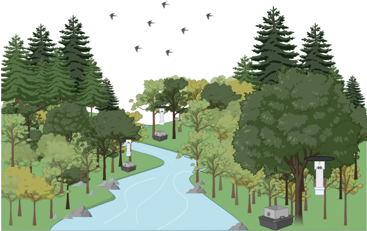
Figure 2. A mock set up of our Mosquito trap array. Every field site had four pairs of a CDC light trap baited with CO 2 and a gravid trap baited with maple leaf infused water. Trap pairs were strategically placed >100 meters away from each other and were in locations that we believed would have high mosquito potential (i.e., in shaded quiet spot). Image created using biorender.com
