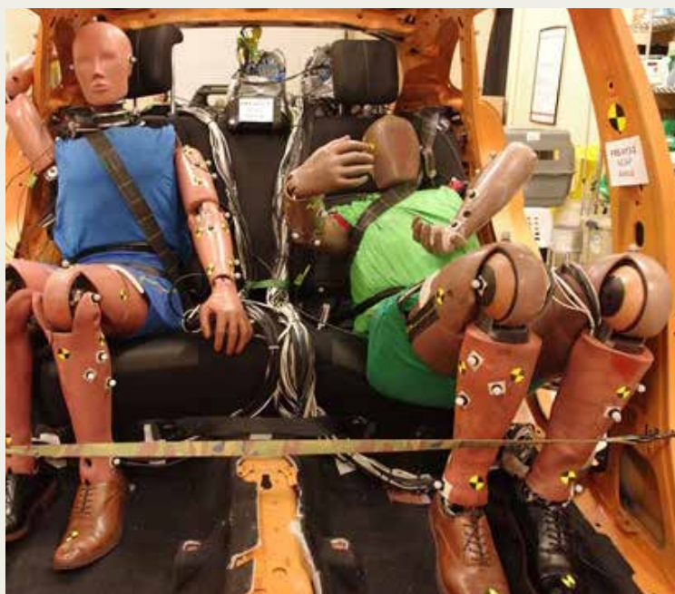
Configurations of the Hybrid III (left) and THOR (right) dummies after an NCAP test on a crash sled. The THOR has slipped under the seatbelt, or "submerged".
