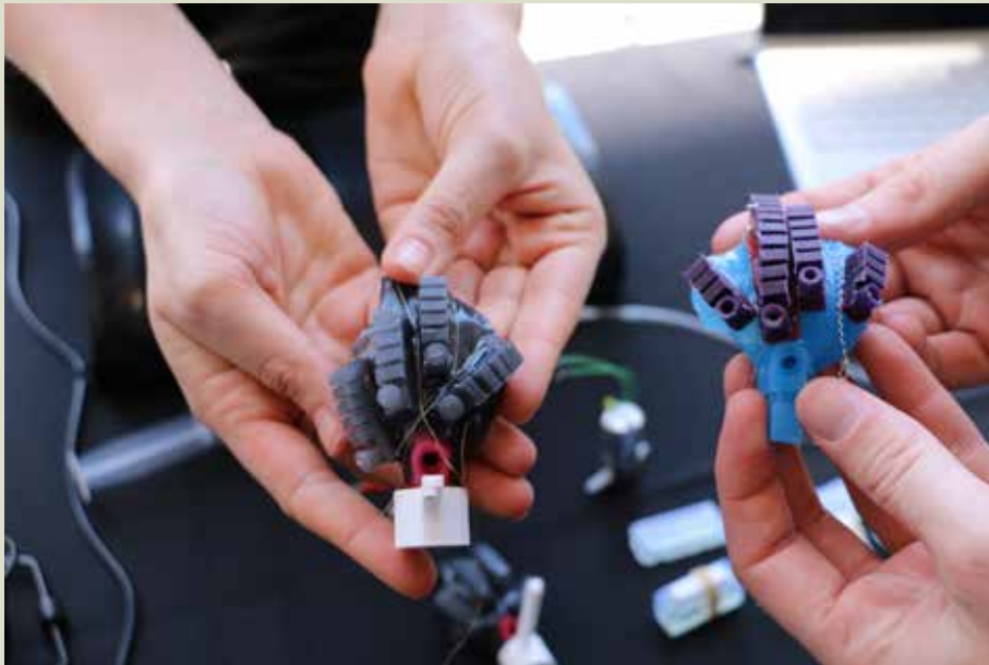
Left: 3-D printed flexible actuators help mimic ear movements on a robotic bat.
